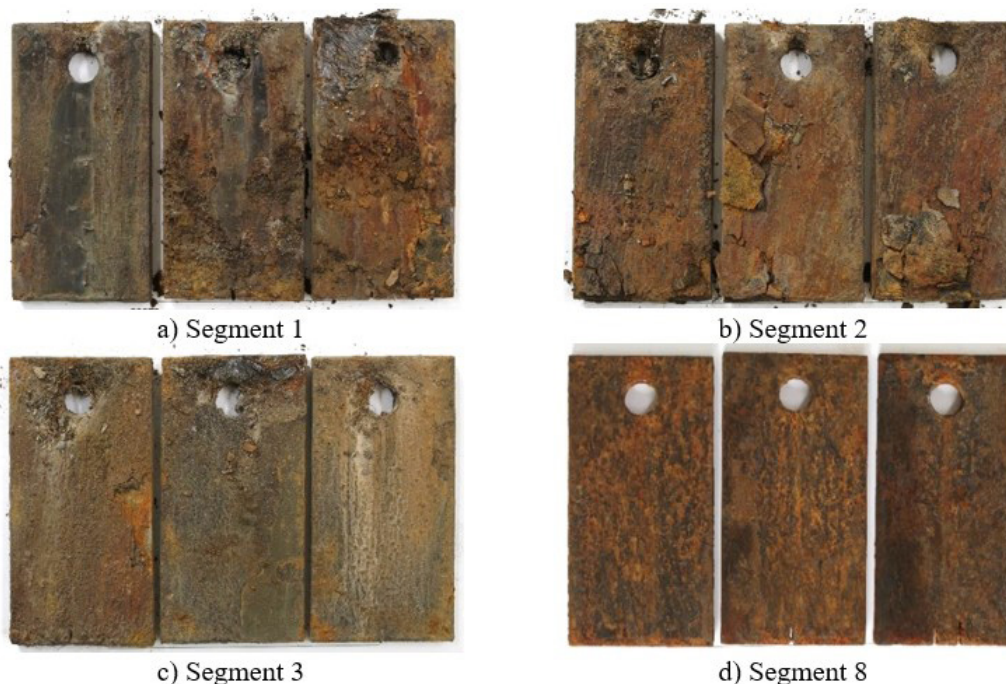
Figure 6. Typical appearance of coupons after corrosion test inside CCM.
