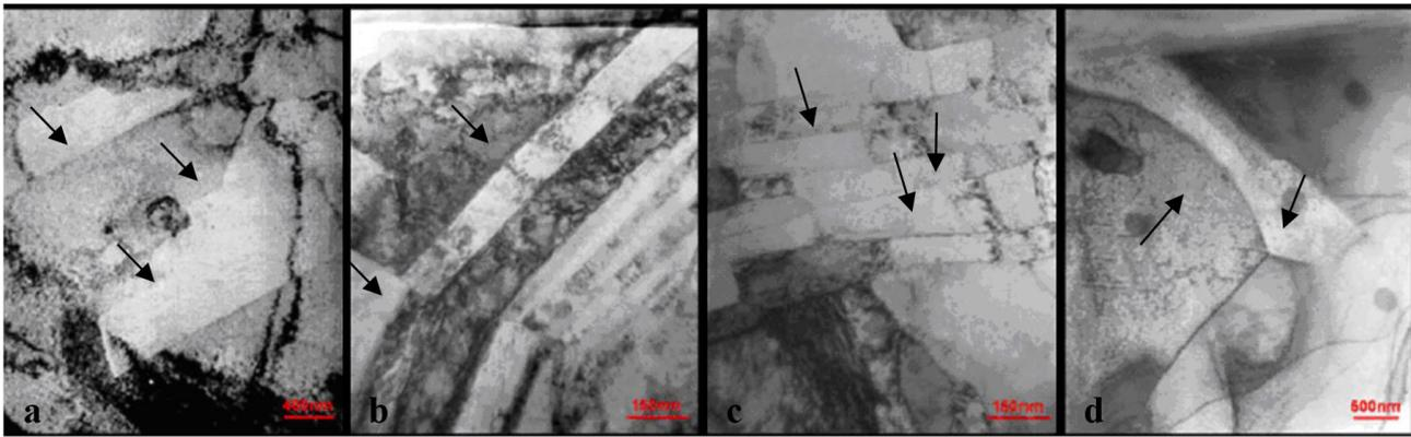
**Figure 2.** TEM micrographs of wires drawn at 77 K to diameters of (a) 5.00 mm ( $\epsilon = 1.30$ ), (b) 4.14 mm ( $\epsilon = 1.68$ ), (c) 3.15 mm ( $\epsilon = 2.23$ ) and (d) 2.02 mm ( $\epsilon = 3.12$ ).
