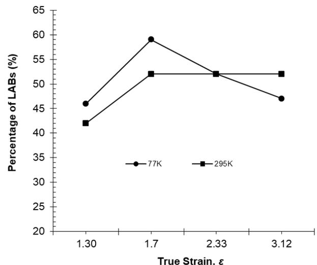
**Figure 4.** Percentage of low-angle boundaries as a function of deformation.
