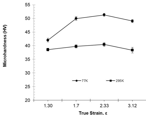
**Figure 5.** Vickers microhardness versus true strain for drawn wires processed at 295 K and 77 K.
