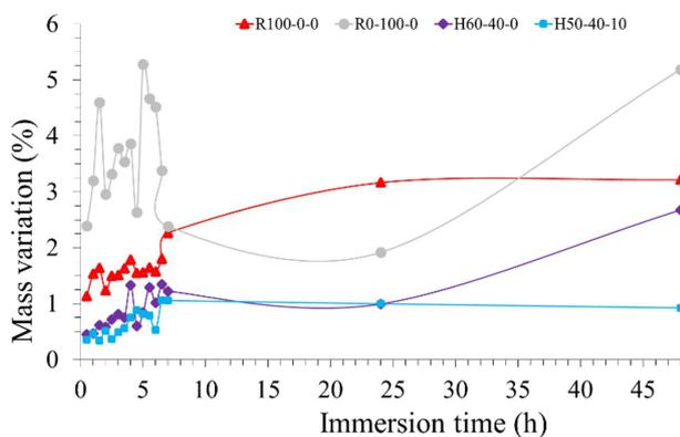
Figure 7. Average water absorption test results.
