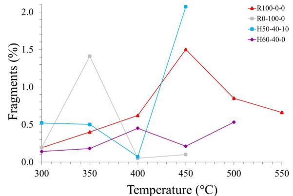
Figure 8. Average briquettes fragments percentage generated at different temperatures.
