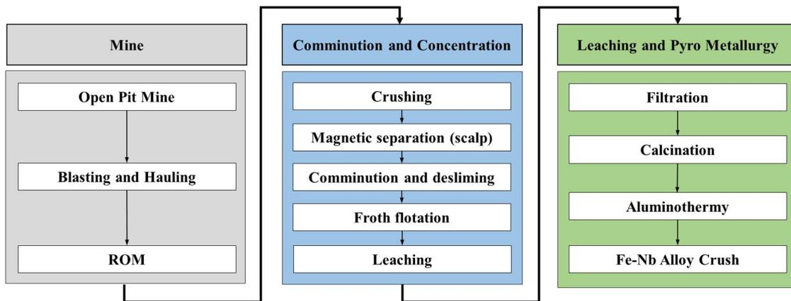
Figure 2. Fe-Nb alloy production flowsheet.
