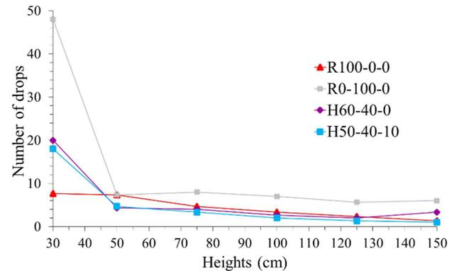
Figure 5. Average shatter test results.
