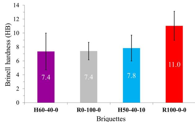
Figure 9. Briquettes average Brinell hardness.
