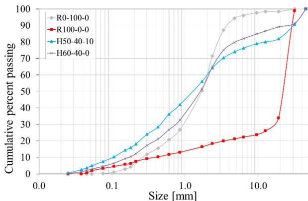
Figure 10. Granulometric analysis of the briquettes after the tumbler test.
