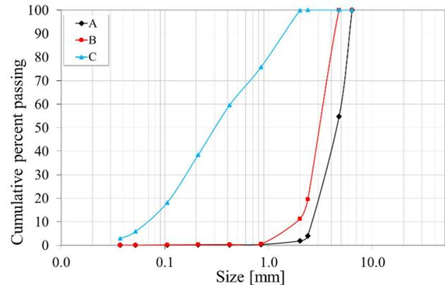
Figure 4. Granulometric analyse of the Fe-Nb fine mixes before the agglomeration. Type A (under 2 mm), type B (between 1 and 5 mm), and type C (between 3 and 15 mm).
