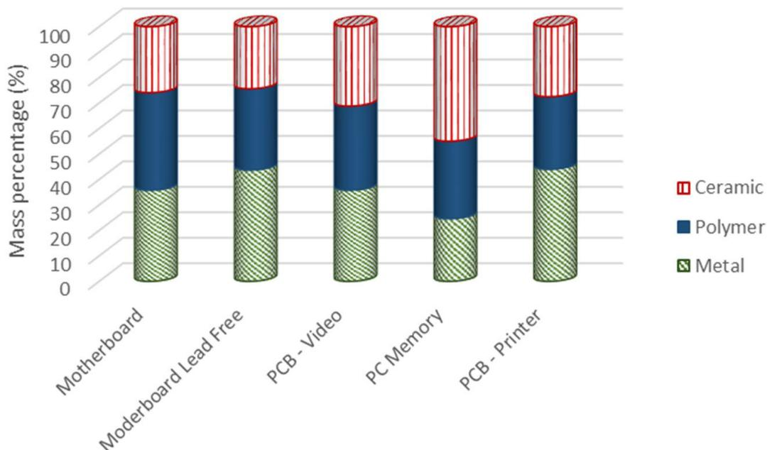
Figure 5. Mass balance of printed circuit boards examined in this study.
