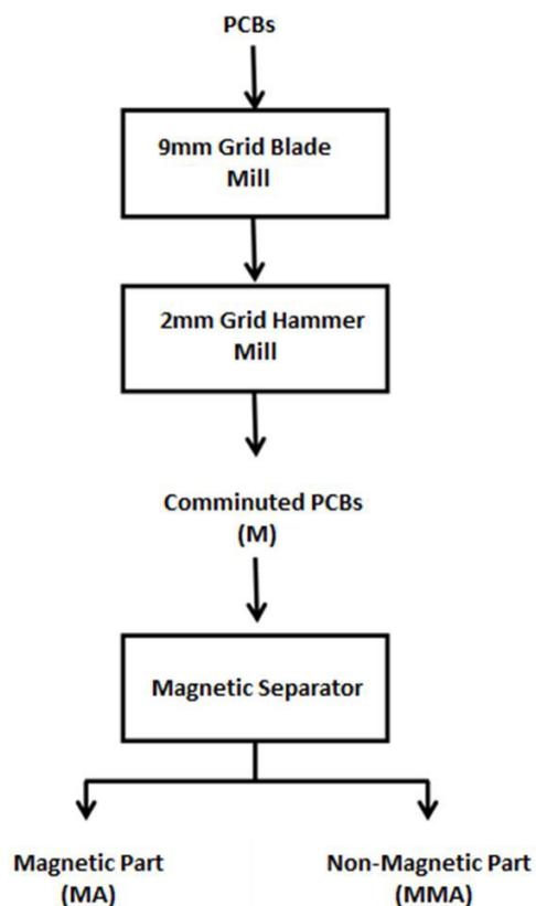
Figure 1. Flowchart of the physical processing of printed circuit boards.
