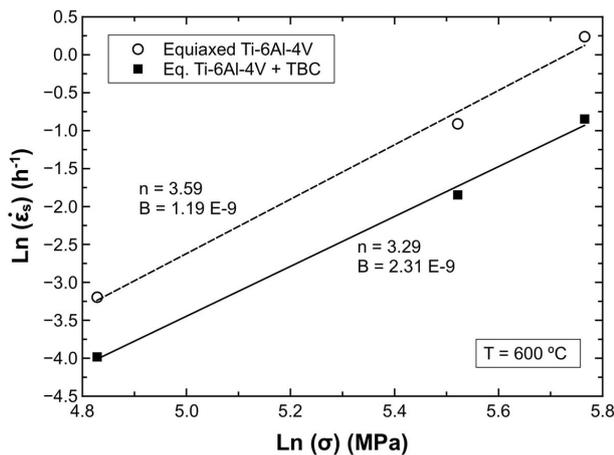
**Figure 3.** Dependence of steady-state rate on applied stress at 600 °C for equiaxed Ti-6Al-4V and Ti-6Al-4V with TBC.
