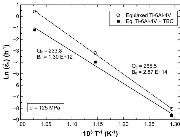
**Figure 4.** Dependence of steady-state rate on temperature at 125 MPa for equiaxed Ti-6Al-4V and Ti-6Al-4V with TBC.
