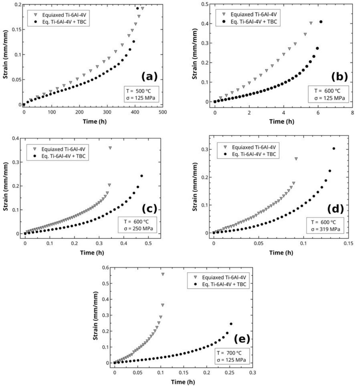
**Figure 2.** Creep curves of equiaxed Ti-6Al-4V and Ti-6Al-4V with TBC at a) 500 °C and 125 MPa; b) 600 °C and 125 MPa; c) 600 °C and 250 MPa; d) 600 °C and 319 MPa; e) 700 °C and 125 MPa.
