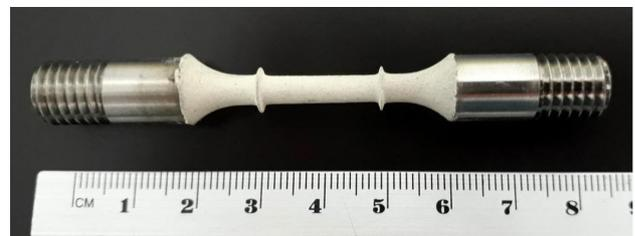
Figure 1. Creep test sample with Thermal Barrier Coating.
