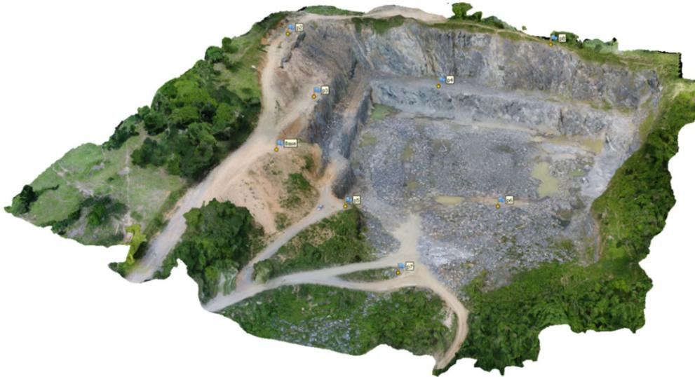
**Figure 3.** Digital Terrain Model (DTM) obtained by Drone Deploy from 80 meters height UAV flight.
