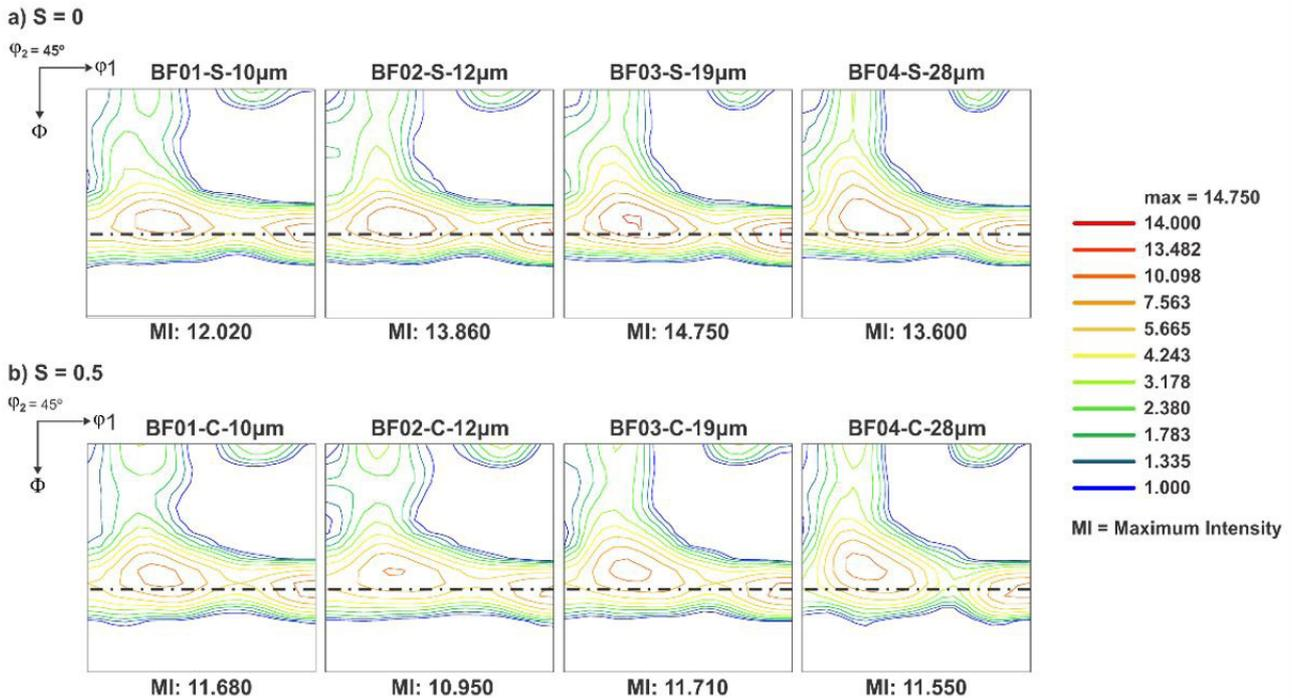
**Figure 3.** Recrystallization textures of the samples, where (a)  $s = 0$  (BFXX-S) represents the surface layer and (b)  $s = 0.5$  (BFXX-C) represents the center layer.
