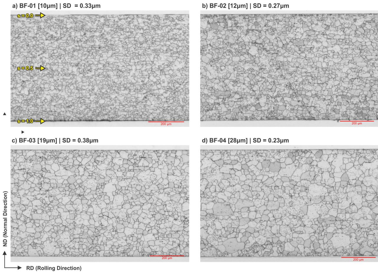
**Figure 1.** Microstructure in 200  $\mu\text{m}$  (red bar) and average grain size of 430Nb samples after the heat treatment. (a) No additional heat treatment; (b) with additional heat treatment of 915°C; (c) with additional heat treatment of 965°C; and (d) with additional heat treatment of 1015°C ( $s = 0$  for surface layer and  $s = 0.5$  for center layer). SD It is an abbreviation for standard deviations.
