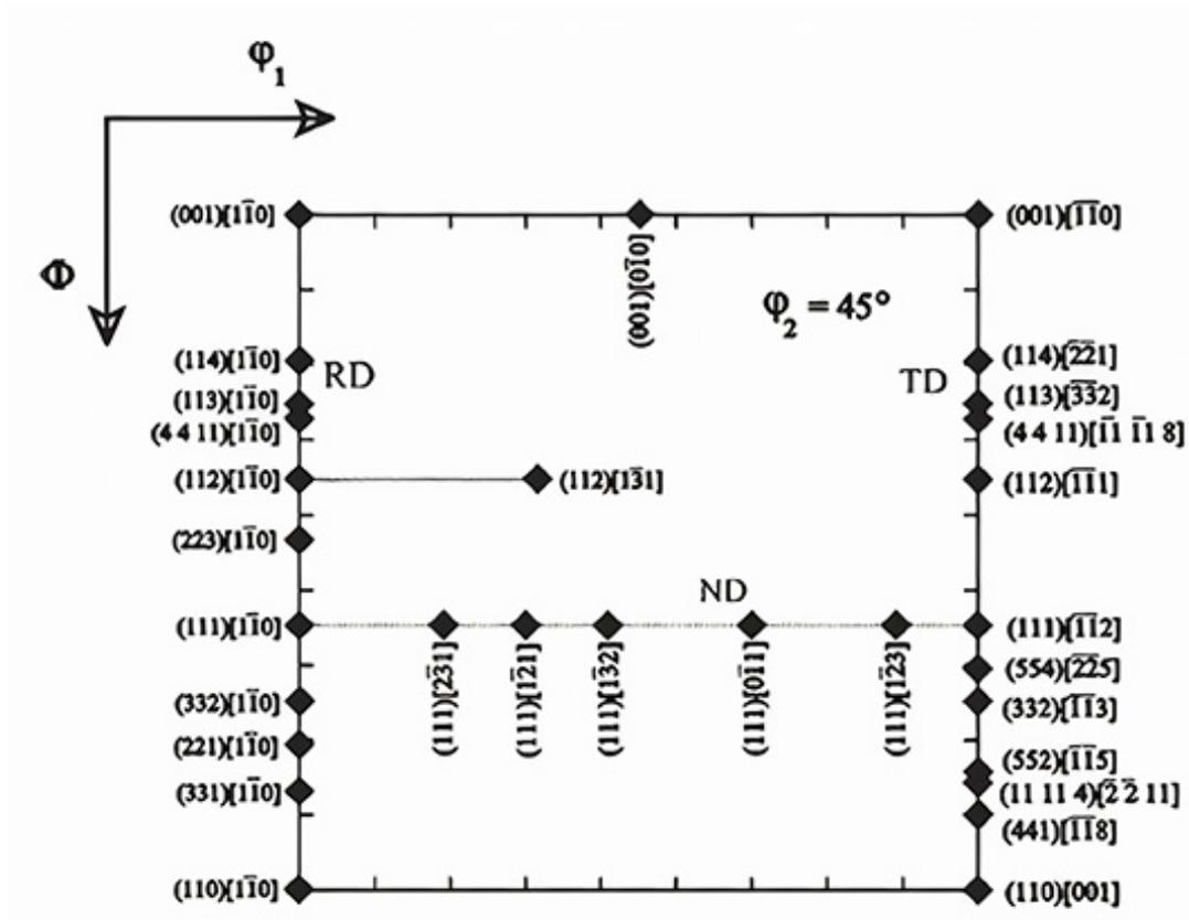
**Figure 2.** Section for  $\delta_2 = 45^\circ$  showing the position of main orientations along with the RD, TD: transverse direction and ND. Euler angles on notations proposed by Bunge [12]
