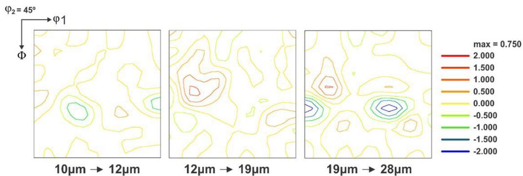
**Figure 4.** Texture change shown by subtraction of ODFs samples in function of grain growth, where (a)  $s = 0$  represents the surface layer and (b)  $s = 0.5$  represents the center layer.
