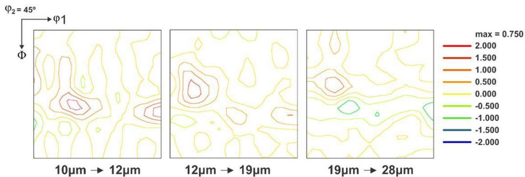
**b) S = 0.5 (CENTER)**
