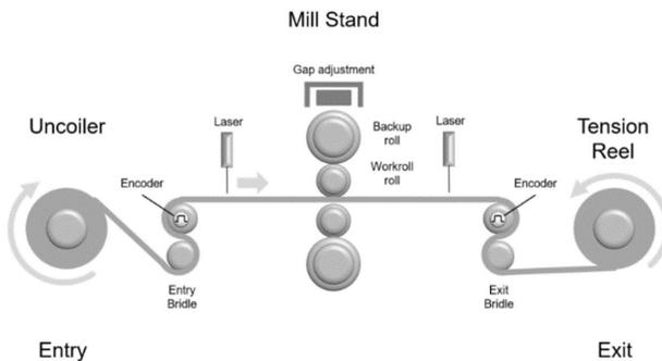
Figure 2. Standard Skin Pass Mill Configuration.
