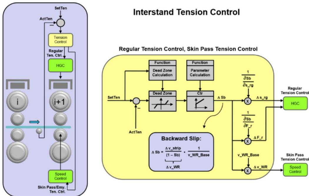
Figure 5. Model Based Inter Stand Tension Control.
