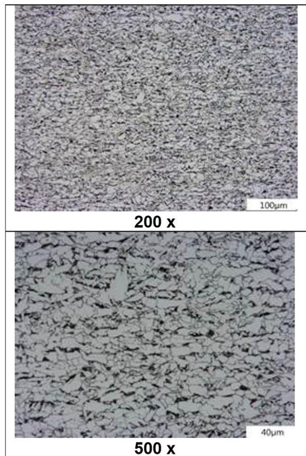
Figure 5. Typical microstructures at  $\frac{1}{4}$  of the thickness of thick 25.40 mm plates. Nital etching 3%.
