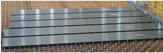
Figure 4. 25.40 mm thick plates in the cooling bed.
