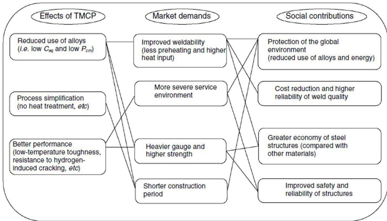
Figure 1. Relationship between market requirements and the roles of thermomechanical treatment [2].
