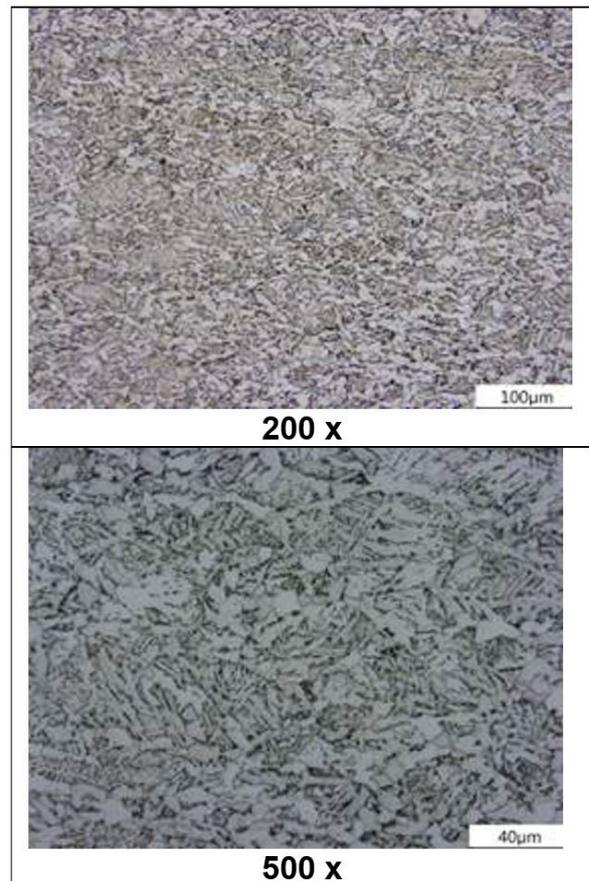
Figure 6. Typical microstructures at  $\frac{1}{4}$  thickness of 50.80 mm thick plates. Nital etching 3%.
