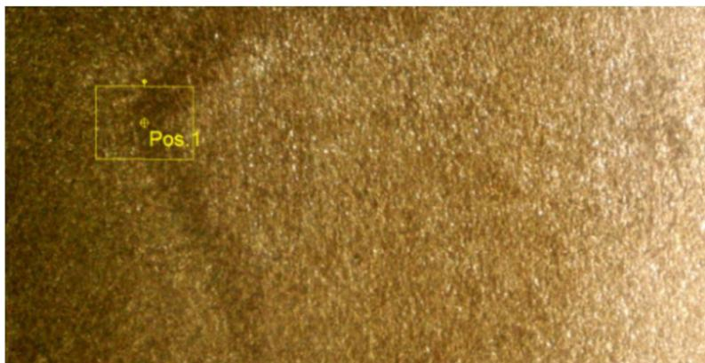
**Figure 11.** Detail of degenerated carbides.
