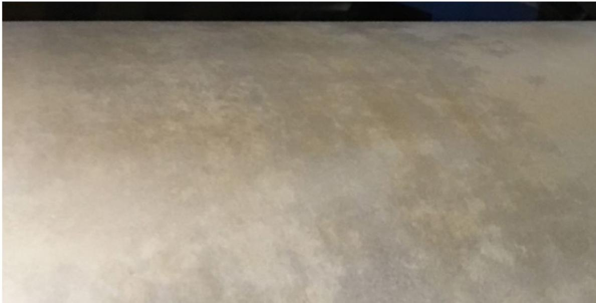
**Figure 15.** Barrel surface with “cloud-pattern”.
