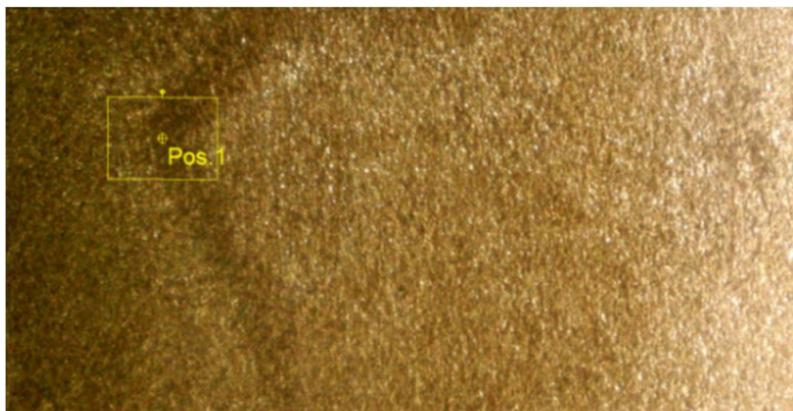
**Figure 11.** Detail of degenerated carbides.
