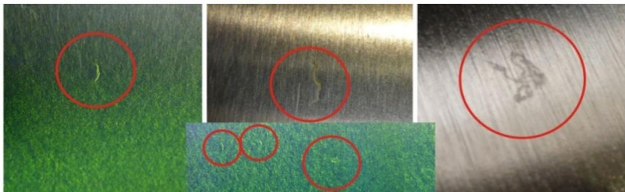
Figure 7. Typical appearance of insufficiently dissolved ferroalloys.
