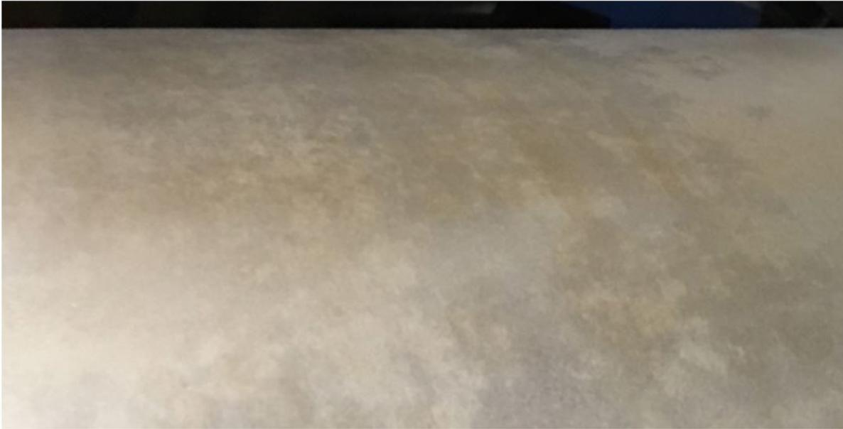
**Figure 15.** Barrel surface with “cloud-pattern”.
