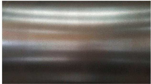
Figure 28. Smooth VANIMO barrel surface without irregularities after rolling a campaign with ~4700 tons.
