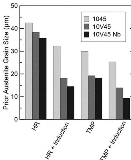
**Figure 3.** Average prior-austenite grain size (PAGS) after hot-rolling or thermomechanical rolling of three 1045 steel variants, and the associated PAGS after simulated induction hardening.
