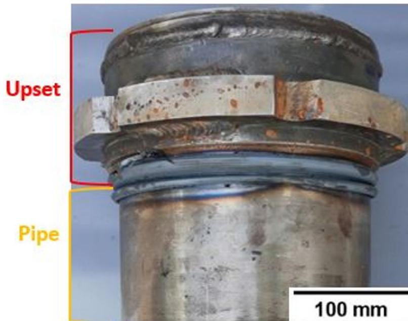
**Figure 6.** Top surface appearance of the welded joint.
