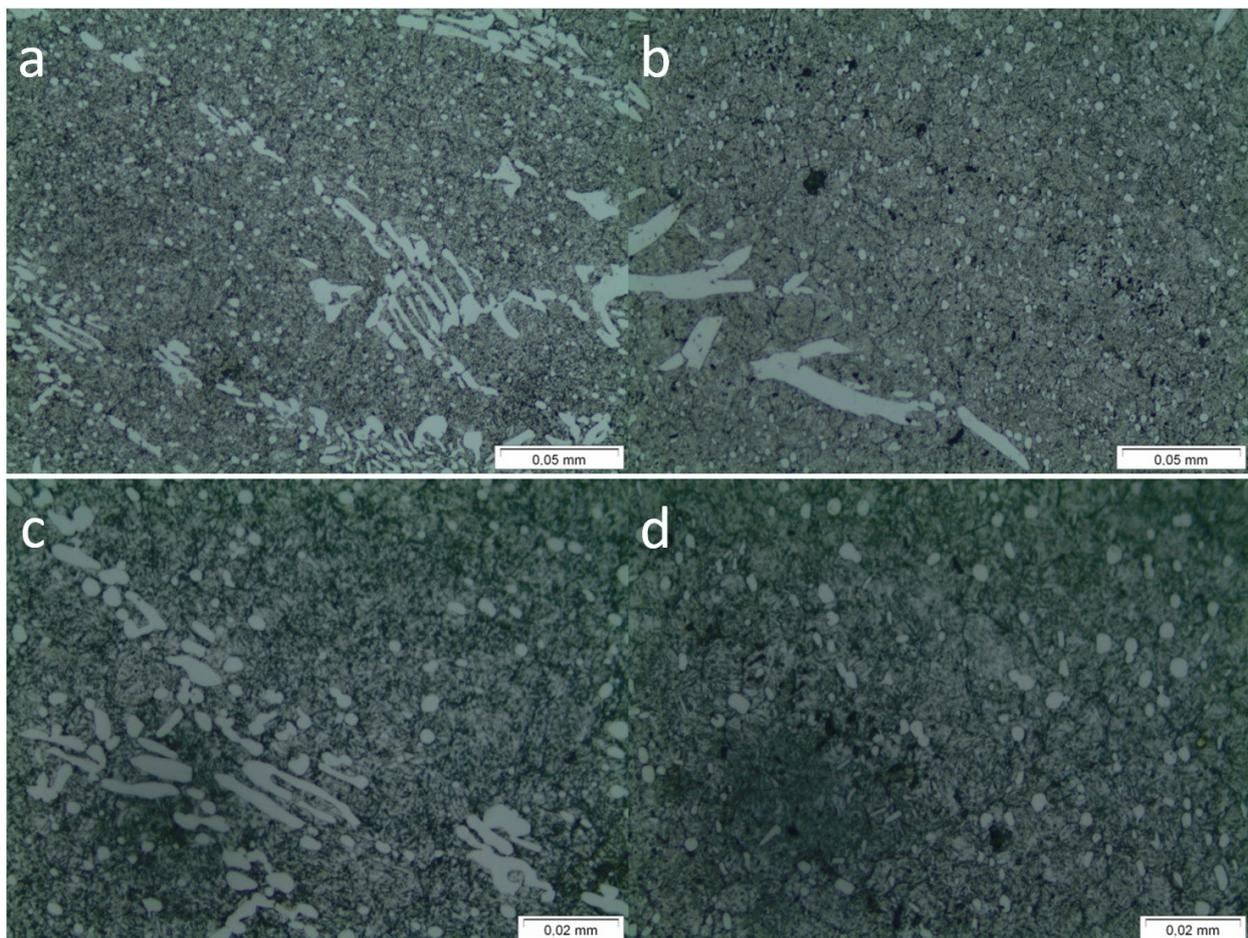
**Figure 3.** Lower magnification photomicrography of (a) CHT samples and (b) DCT sample. Higher magnification photomicrography of (c) CHT samples and (d) DCT sample.
