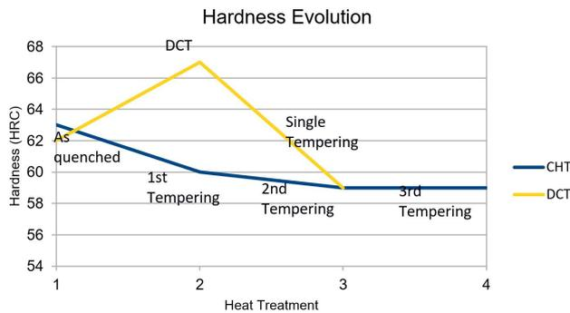
Figure 7. Hardness evolution after CHT and DCT.
