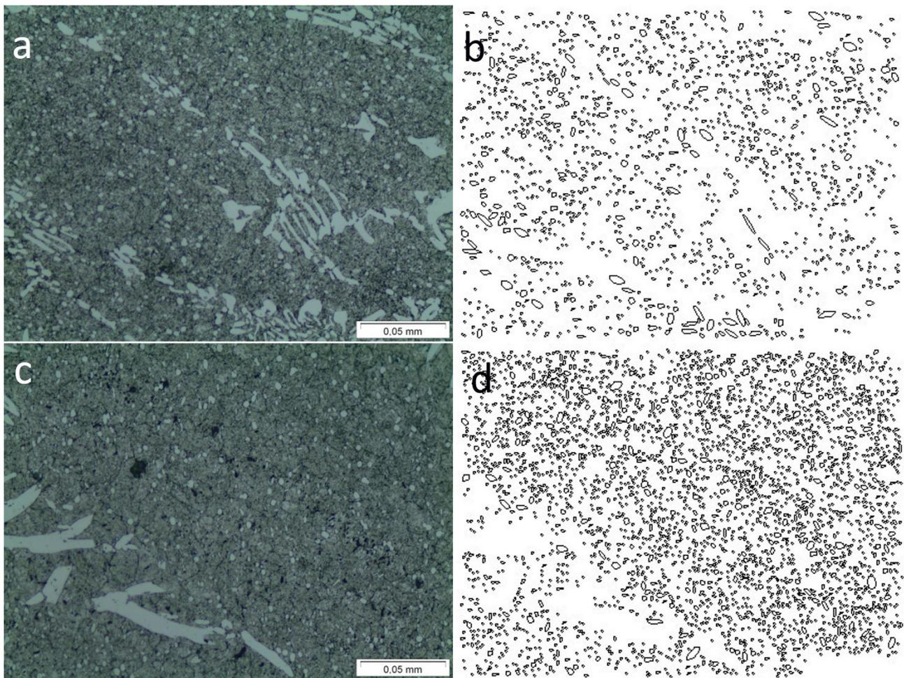
**Figure 4.** Binarization using ImageJ Software. (a) and (b) Sample CHT. (c) and (d) Sample DCT.
