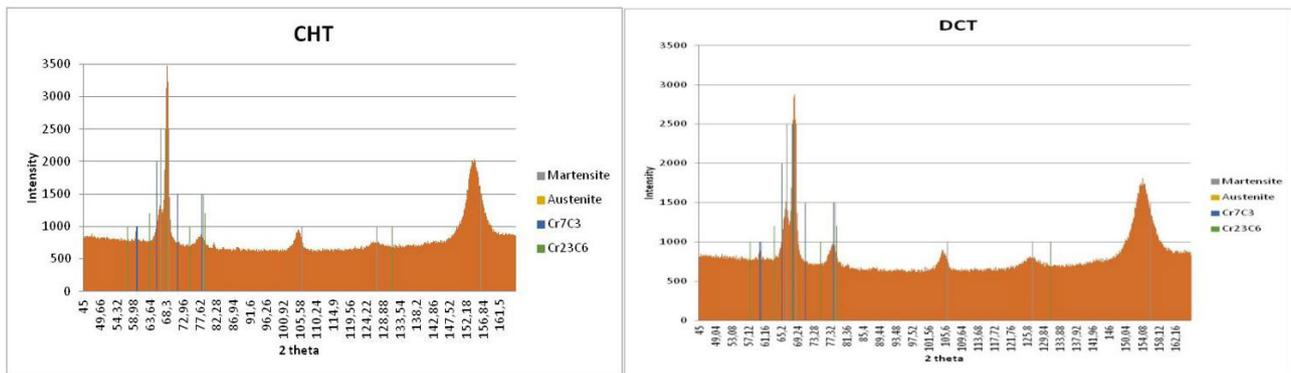
Figure 6. X-ray diffraction for CHT and DCT samples.
