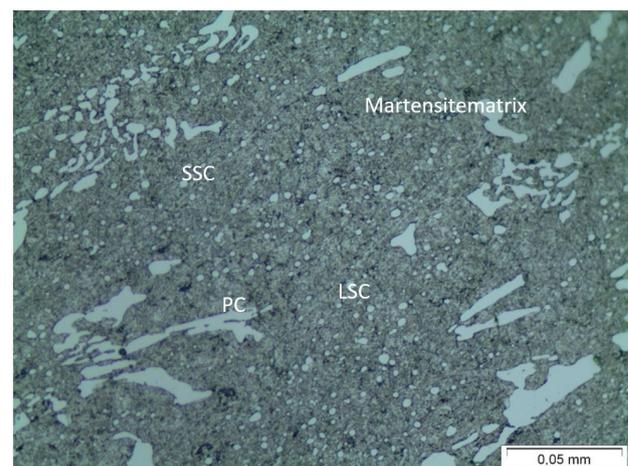
**Figure 2.** Micrograph of CHT sample, where the martensite matrix, PC, SSC and LSC can be observed.
