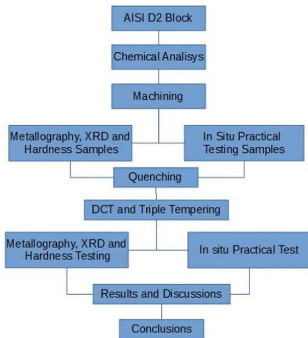
**Figure 1.** Block diagram showing the experimental procedure.
