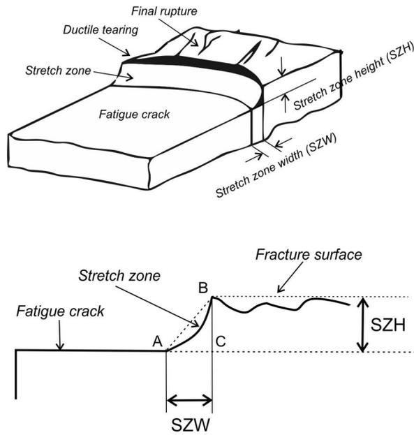
Figure 5. Stretch zone formation (SZW) on a fracture surface.
