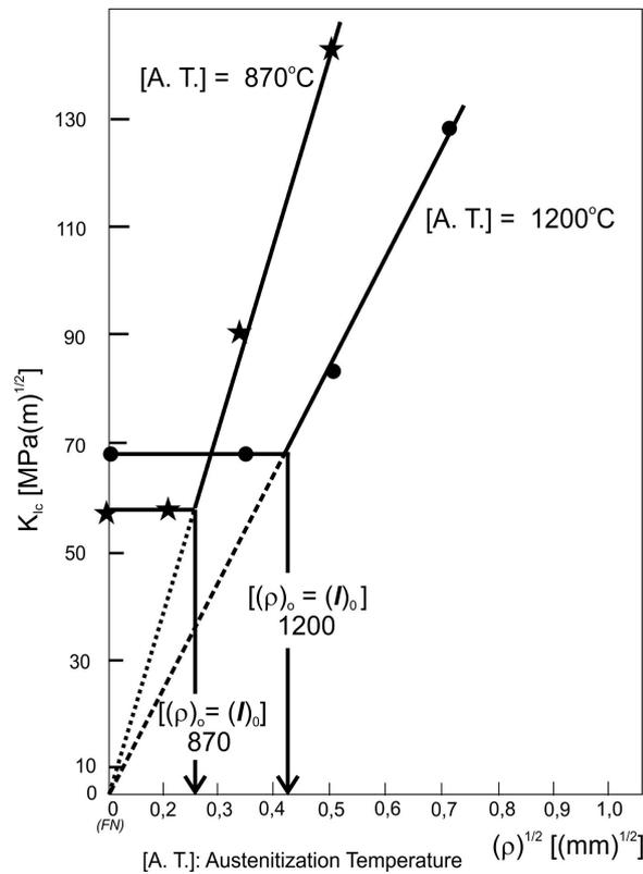
**Figure 2.** Fracture toughness  $K$  values for different crack notch radius for AISI 4140 Quenched steel - A.T. = Austenitization Temperature [48].
