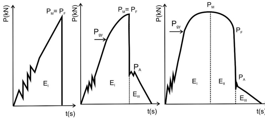
**Figure 3.** Instrumented Charpy test: load – time curves.
