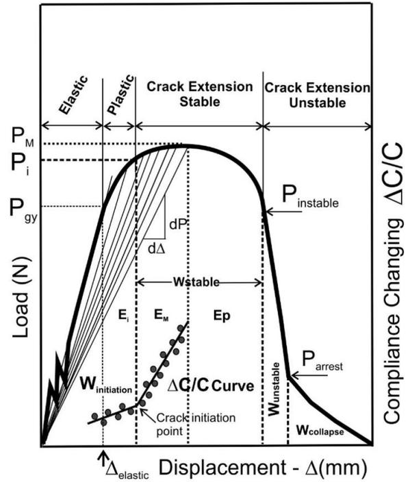
Figure 4. Load - Displacement and Load - Compliance Changing curves.
