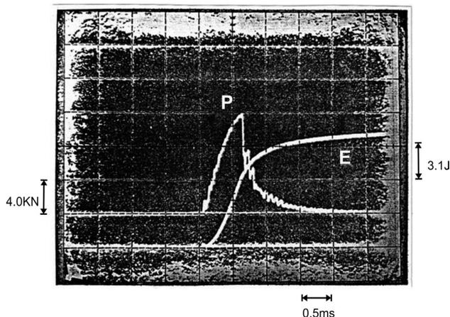
Figure 1. Instrumented Charpy test: Load (P-t) and Energy (E-t) curves.
