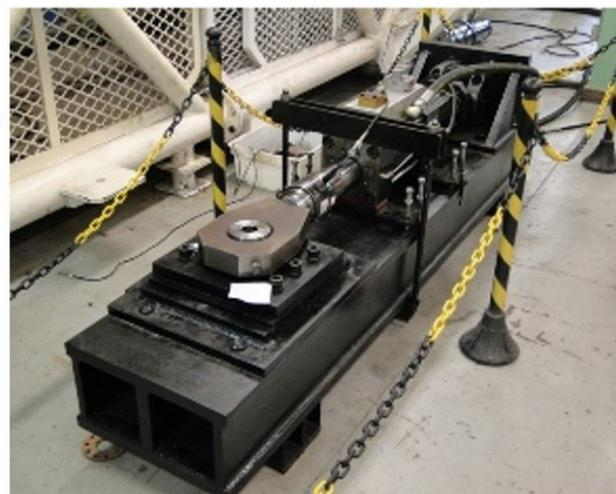
Figure 2. Bench test on kingpin.
