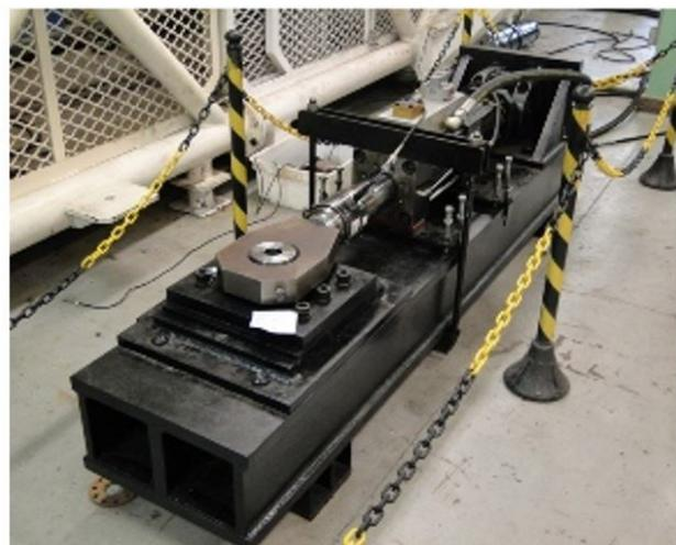
Figure 2. Bench test on kingpin.
