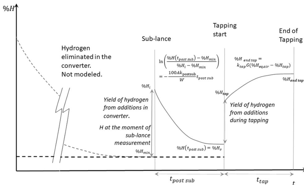
**Figure 4.** Schematic evolution of hydrogen in the steelmaking process, according to the formulated model. See text for discussion.
