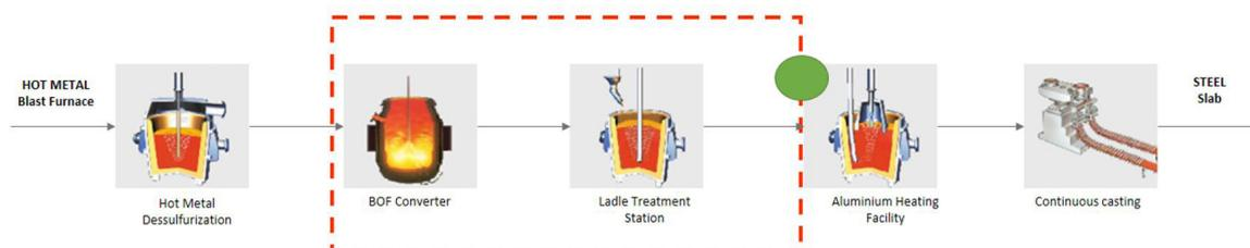
**Figure 2.** Steel production flow for a non-vacuum treated steel at Ternium, highlighting steps considered in this study. The green dot indicates the point where H is currently measured at Ternium, to decide if the heat must be degassed for casting safety.
