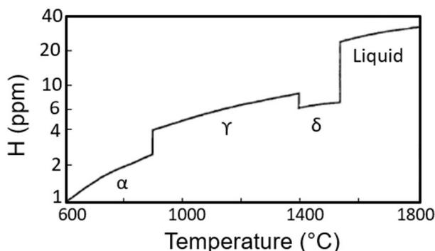
**Figure 1.** Solubility of hydrogen in iron (and low alloy steels) at 1 atm as a function of temperature. Adapted from Turkdogan [1].
