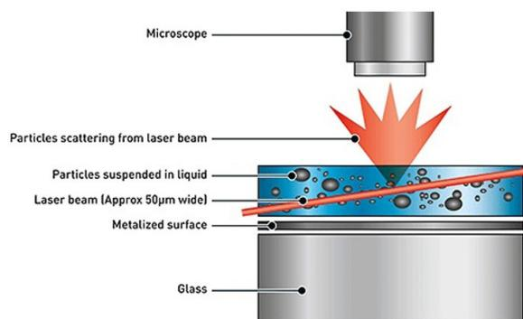
**Figure 2.** Principle of operation of the NTA-LM20 equipment used in this study.
