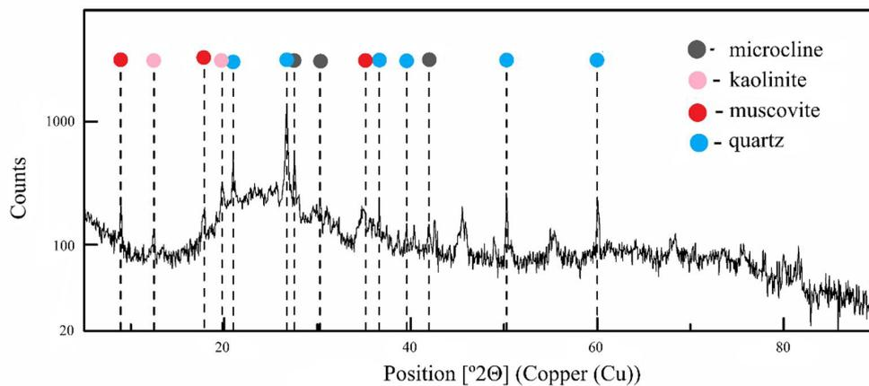
**Figure 4.** X-ray diffraction pattern of metakaolin (MK).
