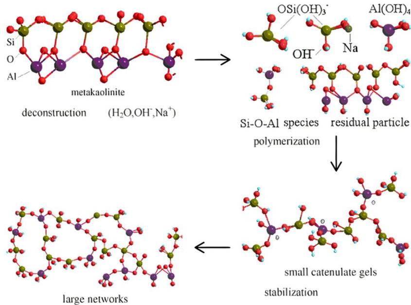
**Figure 2.** Sketch of the geopolymerization process, including the deconstruction of metakaolinite (MK) by alkalination, the polymerization of generated alumina/silica-hydroxy species and the stabilization of fresh formed structures [10].
