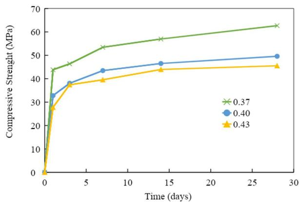
**Figure 6.** Compressive strength (MPa) x time (days) of 3 tests varying W/S ratio.
