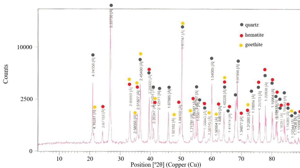
**Figure 5.** X-ray diffraction pattern of iron ore tailings (IOT).
