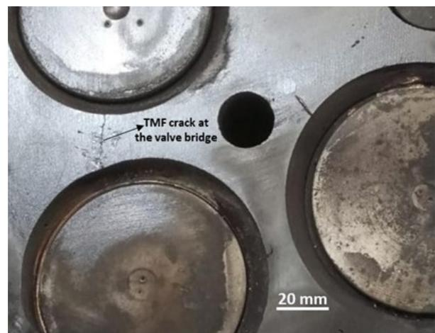
**Figure 1.** Failed cylinder head due to TMF process. It is observed a crack (arrow) at the valves bridge. Picture taken in a Brazilian automotive workshop.
