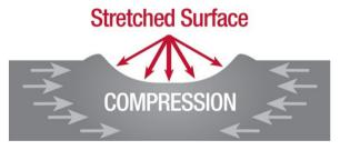
Figure 6. Schematic illustration of the surface after shot peening [16].
