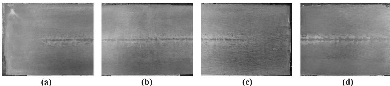
**Figure 4.** BW AC C77MD representative macro etching photographs, transversal (a) left side, (b) right side, (c) middle, and (d) longitudinal.
