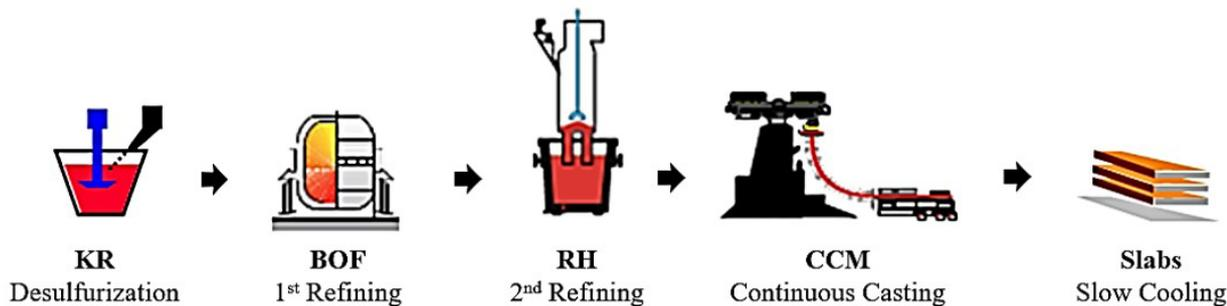
Figure 2. Slab production stream at ArcelorMittal Tubarão to guarantee low inclusion levels.
