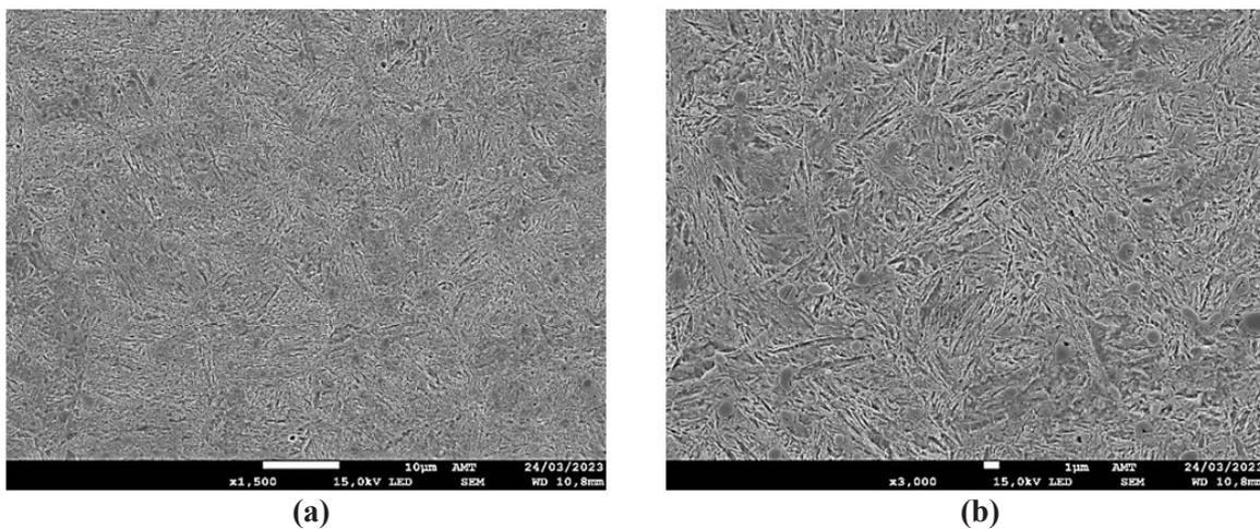
Figure 10. Micrographs of Clutch bearing ring sample after Quenching and Tempering, (a) 1500x and (b) 3000x. SEM – SE – Nital 2%.
