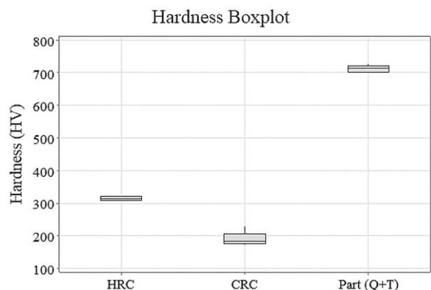
Figure 11. Hardness Boxplot for BW AC C77MD tested samples.
