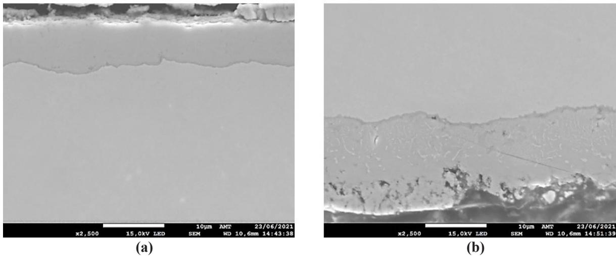
**Figure 7.** Micrographs of Hot Rolled sample near the surface, 2500x, (a) Topside and (b) Bottom side. SEM – SE – No etchant.
