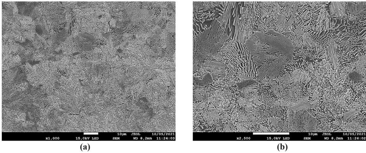
**Figure 6.** Micrographs of Hot Rolled sample, (a) 1000x and (b) 2500x. SEM – SE – Nital 2%.
