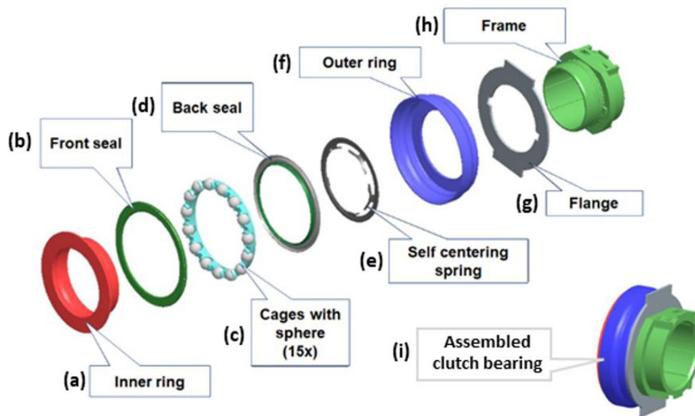
**Figure 1.** An exploded view of the clutch bearing shows: (a) inner ring; (b) front seal; (c) cage with spheres; (d) back seal; (e) self-centering spring; (f) outer ring; (g) flange; and (h) frame. (Provided by Schaeffler).
