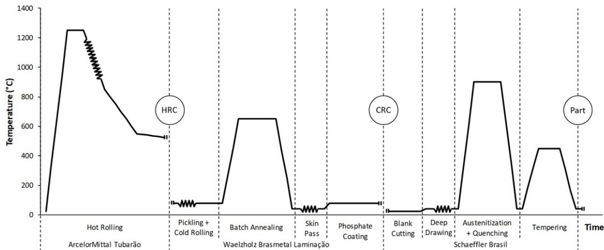
Figure 3. BW AC C77MD steel thermomechanical process stream for clutch bearing ring production.
