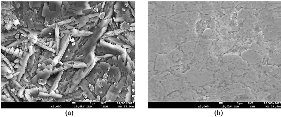
Figure 9. Micrographs of cold-rolled sample surfaces (a) with and (b) without zinc phosphate coating. 3000x. SEM – SE – No etchant.
