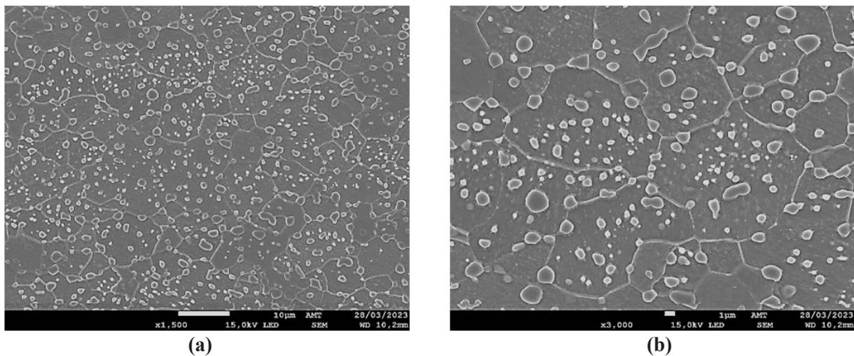
**Figure 8.** Micrographs of Cold Rolled sample, (a) 1500x and (b) 3000x. SEM – SE – Nital 2%.
