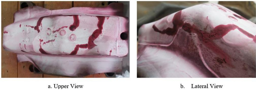
Figure 3. Photographic record of the liquid penetrant analysis of the hot stamping die at the end-of-life.
