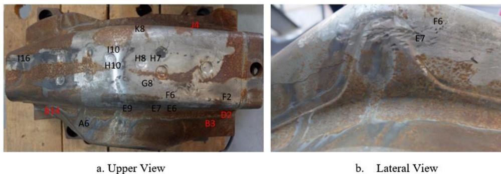
**Figure 2.** Photographic record of the naked eye analysis of the hot stamping die at the end-of-life.
