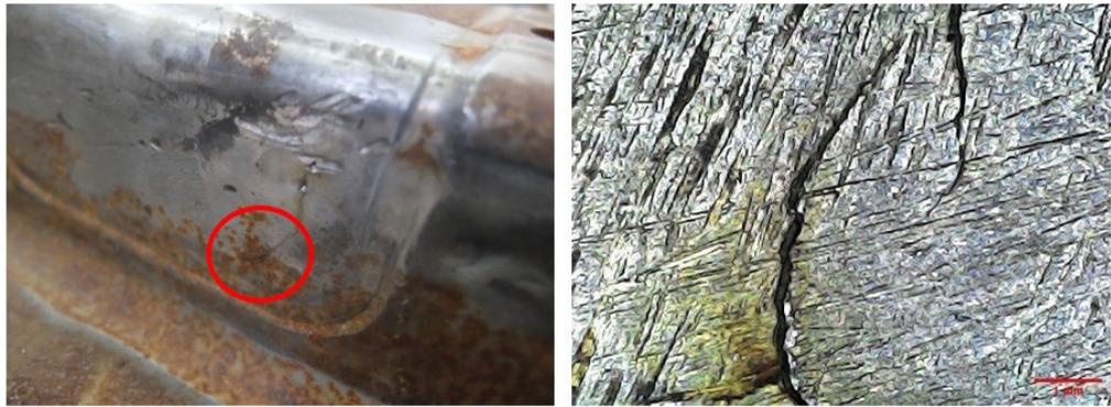
Figure 4. Photograph (left) and photomicrograph (right) of the end-of-life die at position D2. Cracks can be clearly observed.
