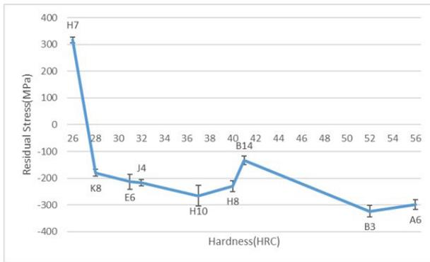
**Figure 13.** Graph of residual stress (MPa) X hardness (HRC).
