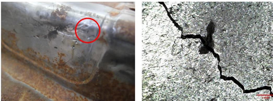
**Figure 11.** Photograph (left) and photomicrograph (right) of the end-of-life die position F2, pulling out, cracks.
