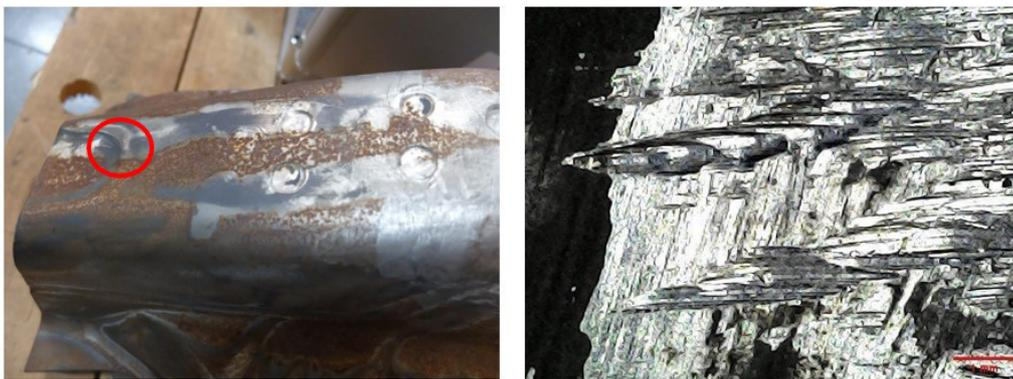
**Figure 7.** Photograph (left) and photomicrograph (right) of the end-of-life die at position I16. Grooves.
