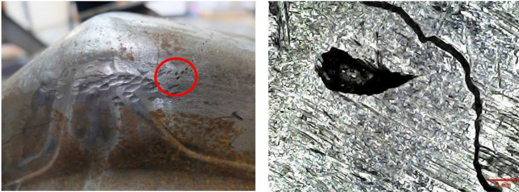
**Figure 6.** Photograph (left) and photomicrograph (right) of the end-of-life die at position F6. Material pulled out, and cracks.
