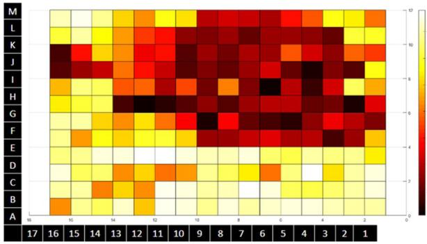
**Figure 12.** End-of-life hot stamping die HRC hardness map, the brighter the higher the hardness.
