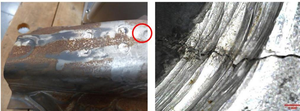
**Figure 8.** Photograph (left) and photomicrograph (right) of the end-of-life die at position I10, cracks.
