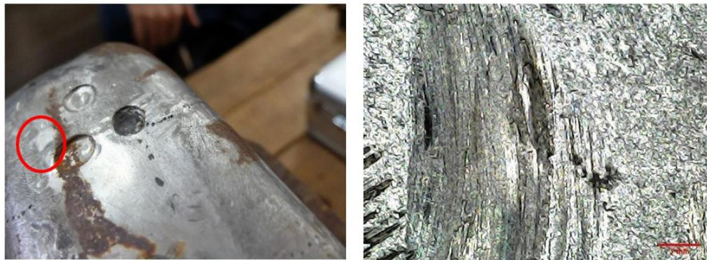
Figure 5. Photograph (left) and photomicrograph (right) of the end-of-life die at G8 position. Grooves in the material flow direction can be seen.
