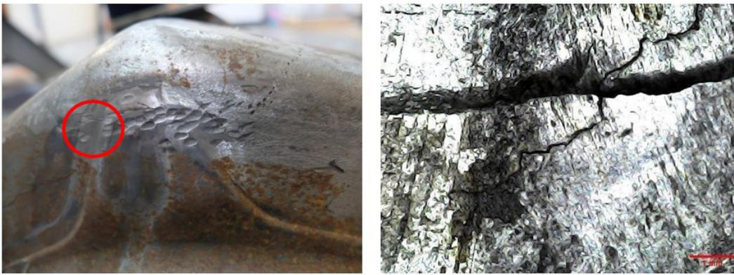
**Figure 10.** Photograph (left) and photomicrograph (right) of the end-of-life die at position E9, cracks.
