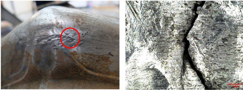
**Figure 9.** Photograph (left) and photomicrograph (right) of the end-of-life die at position E7. Kneading, evidence of impact wear, and cracks.
