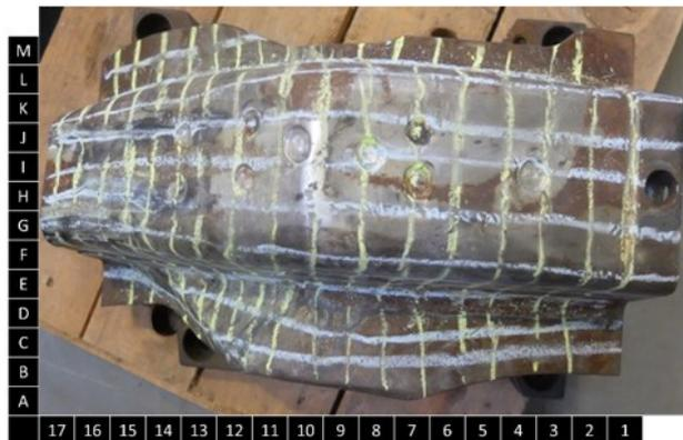
**Figure 1.** Mesh with the identification of the analyzed regions in the end-of-life die for hot stamping process.
