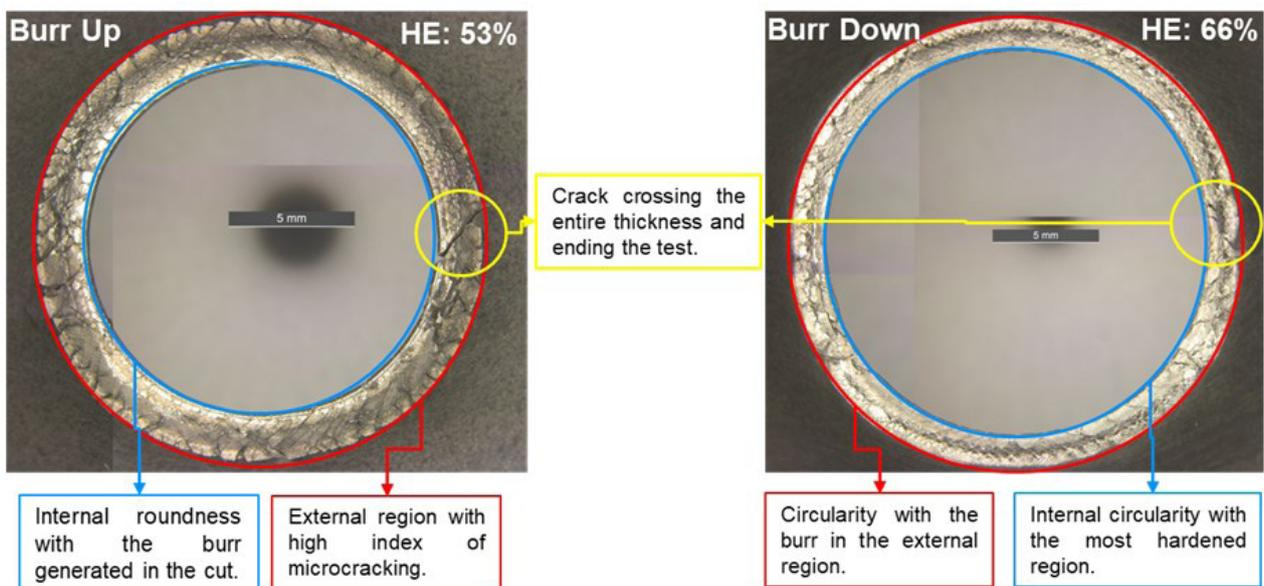
**Figure 9.** Evaluation of the edge generated by punch cutting (Burr Up and Burr Down) after the hole expansion test.
