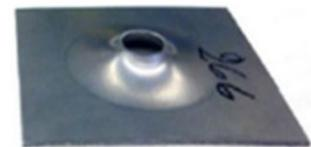
**Figure 5.** Representation of Hole Expansion Test [2].
