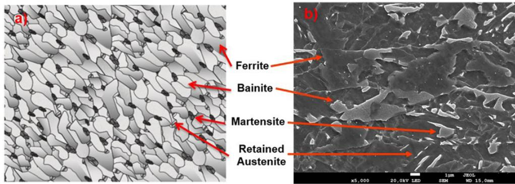
**Figure 1.** a) Scheme of a complex-phase steel microstructure showing martensite and austenite retained in a ferrite-bainite matrix. b) Microstructure of CP800 observed in SEM after Nital 2% attack.
