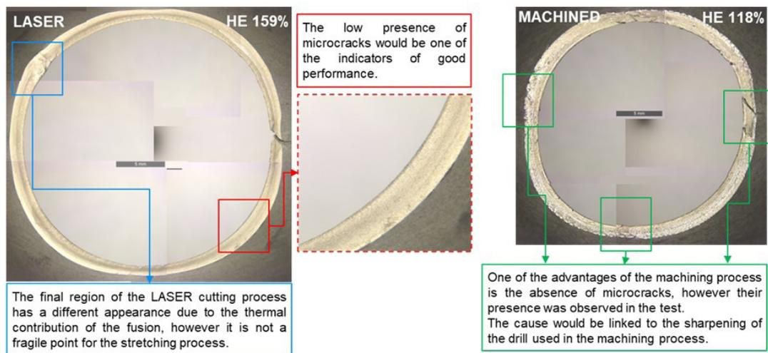
**Figure 12.** Evaluation of the edge generated by LASER and Drilling cuts after the hole expansion test.
