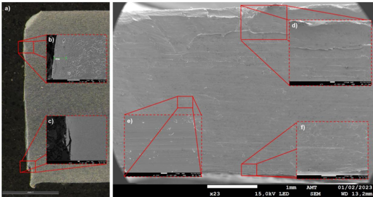
**Figure 11.** Machining cut evaluation. a) Image of the cut profile observed in the stereoscope; b) presence of regions with a certain level of hardening; c) formation of “teeth” on the cutting edge; d) Machining flaws observed on the cutting edge; e) region with good cutting finish and formation of marks parallel to the surface of the material and f) region with low burr level.
