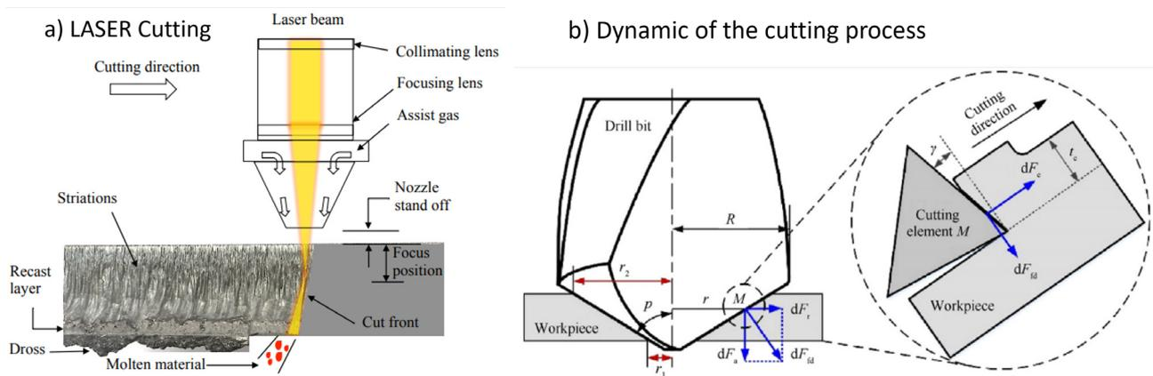
**Figure 4.** Representation of making the hole by LASER and drilling cutting. a) Schematic of the mechanisms during LASER cutting [8] and b) Representation of making the hole by Drilling cutting [9].
