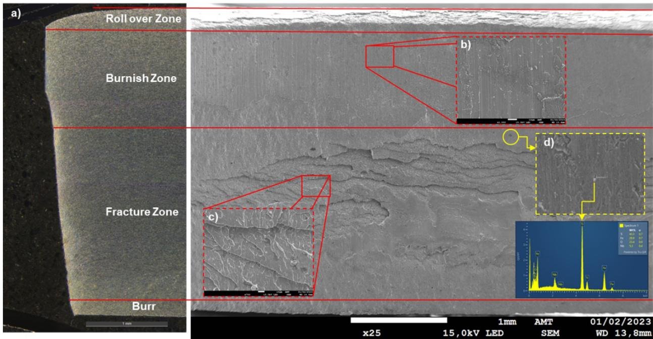
**Figure 8.** Evaluation of the punch cut. a) Image of the cut profile observed in the stereoscope; b) Cut marks in the direction of the punch; c) formation of flaws on the surface due to the high load of the cut; d) observing the presence of a titanium nitride on the cutting edge.
