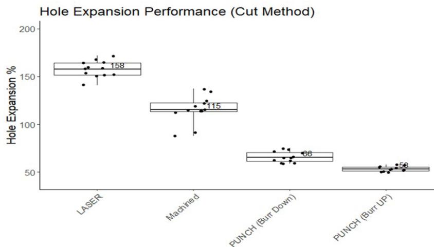
**Figure 7.** Results of HE tests for different cutting methods.
