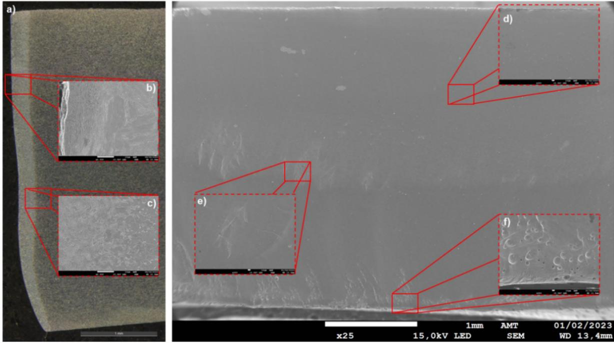
**Figure 10.** Evaluation of LASER cut. a) Image of the cut profile observed in the stereoscope; b) formation of the high hardness martensite constituent; c) the thermal input generated an HAZ of around 250µm; d) region with excellent cutting finish; e) marks of the hot cut with the shape of dendrites and f) presence of bubbles in the region of the end of the cut due to the melting of the material.
