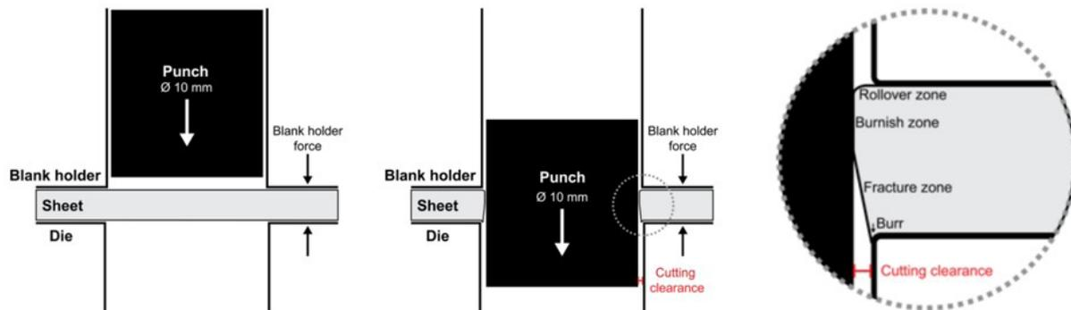
**Figure 2.** Schematic representation of regions normally formed on a cut edge surface [2].
