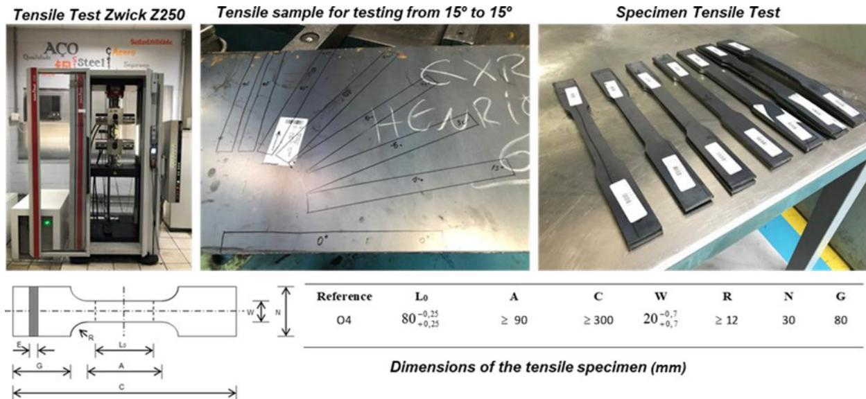
**Figure 3.** Duplicate tensile tests with angle variation every 15° to study hardening (n) and anisotropy (r) properties and coefficients.
