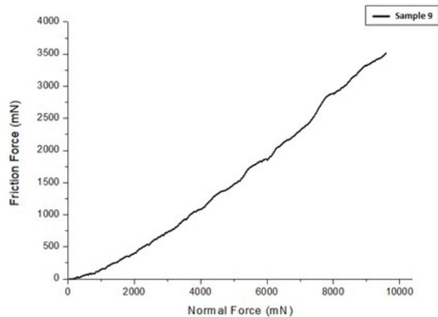
**Figure 4.** Curves of Friction Force × Normal Force obtained during the scratching test of sample 9.
