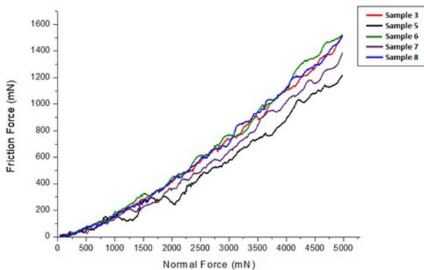
**Figure 3.** Curves of Friction Force × Normal Force obtained during the scratching test of samples 3, 5, 6, 7 and 8.
