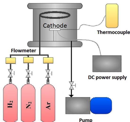
**Figure 1.** Schematic drawing of nitriding system – adapted [12].
