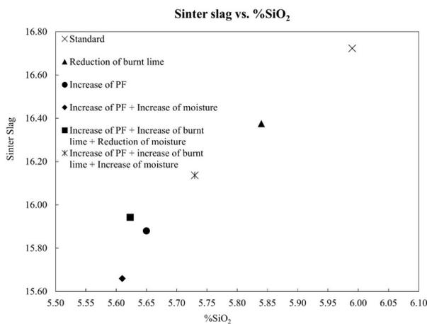
Figure 3. Sinter slag versus silica content in sinter product.
