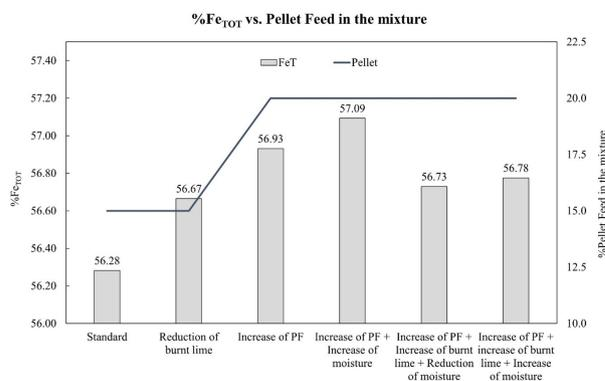
**Figure 2.** Comparison between total iron on sinter product.
