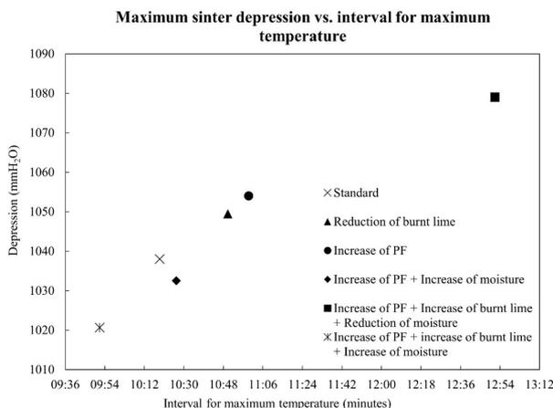
Figure 4. Sintering depression at maximum sintering temperature versus time to achievement of the maximum sintering temperature.
