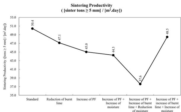
Figure 8. Calculated sintering productivity based on the sinter pot tests.
