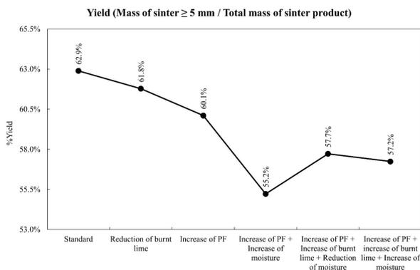
Figure 5. Sinter product yields – percentage of sinter product higher than 5 mm.
