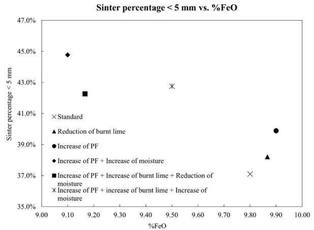
Figure 6. The relation between the percentage of fines in the sintered product (percentage lower than 5 mm for the sinter pot tests) and %FeO in the sintered product.
