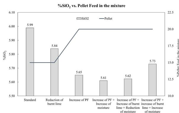
**Figure 1.** Comparison of silica content in sinter product between the standard operational practice and other investigation lines, considering mainly the increase of pellet feed in the sintering mixture.
