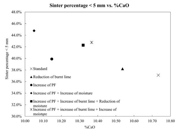
Figure 7. The relation between percentage of fines in sinter product (percentage lower than 5 mm for the sinter pot tests) and %CaO in the sinter product.
