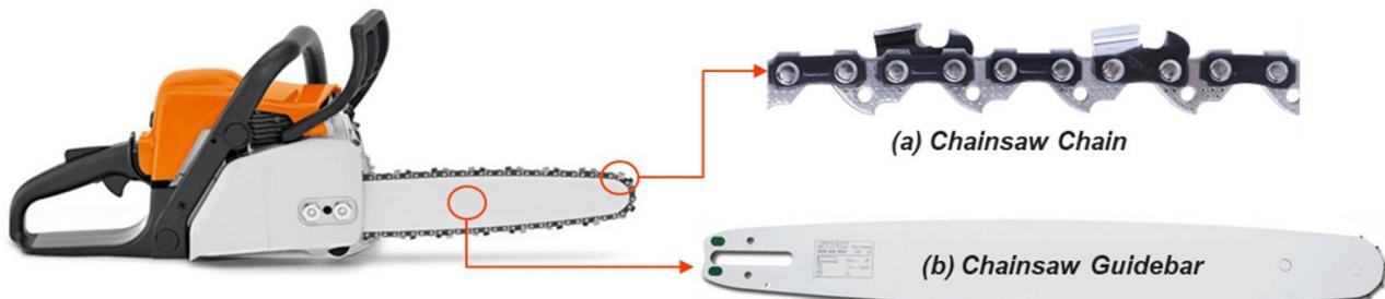
Figure 1. Chainsaws are composed of different steel parts, such as the chain (a) and the bar (b), which are the focus of the study.
