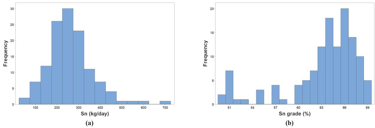
Figure 9. Frequency histogram of the daily Sn production (a) and grade (b) for the jigs and shaking tables combined plants.
