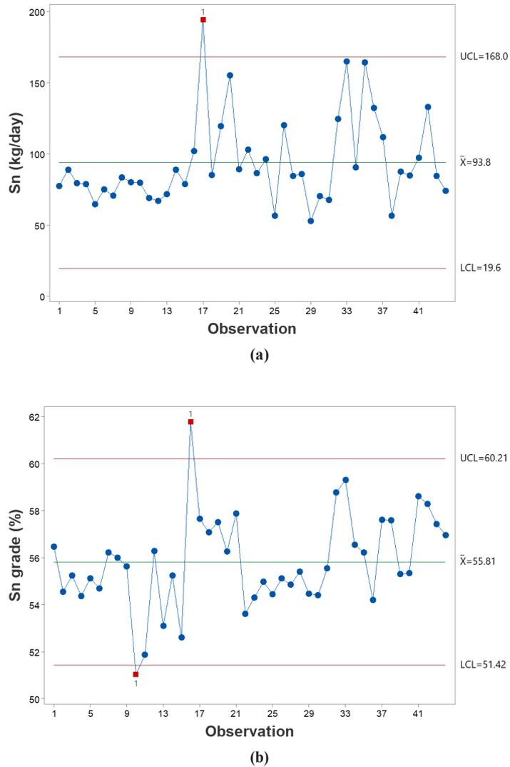
Figure 7. Control chart of the daily Sn production (a) and grade (b) for one shaking table.
