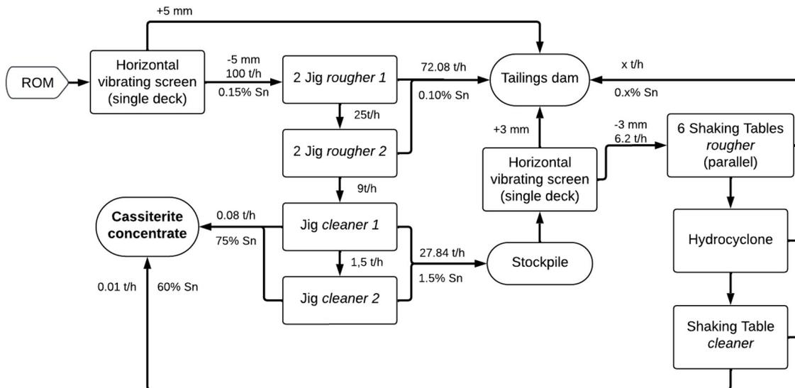
Figure 8. Optimized cassiterite processing flowsheet with the shaking tables plant.
