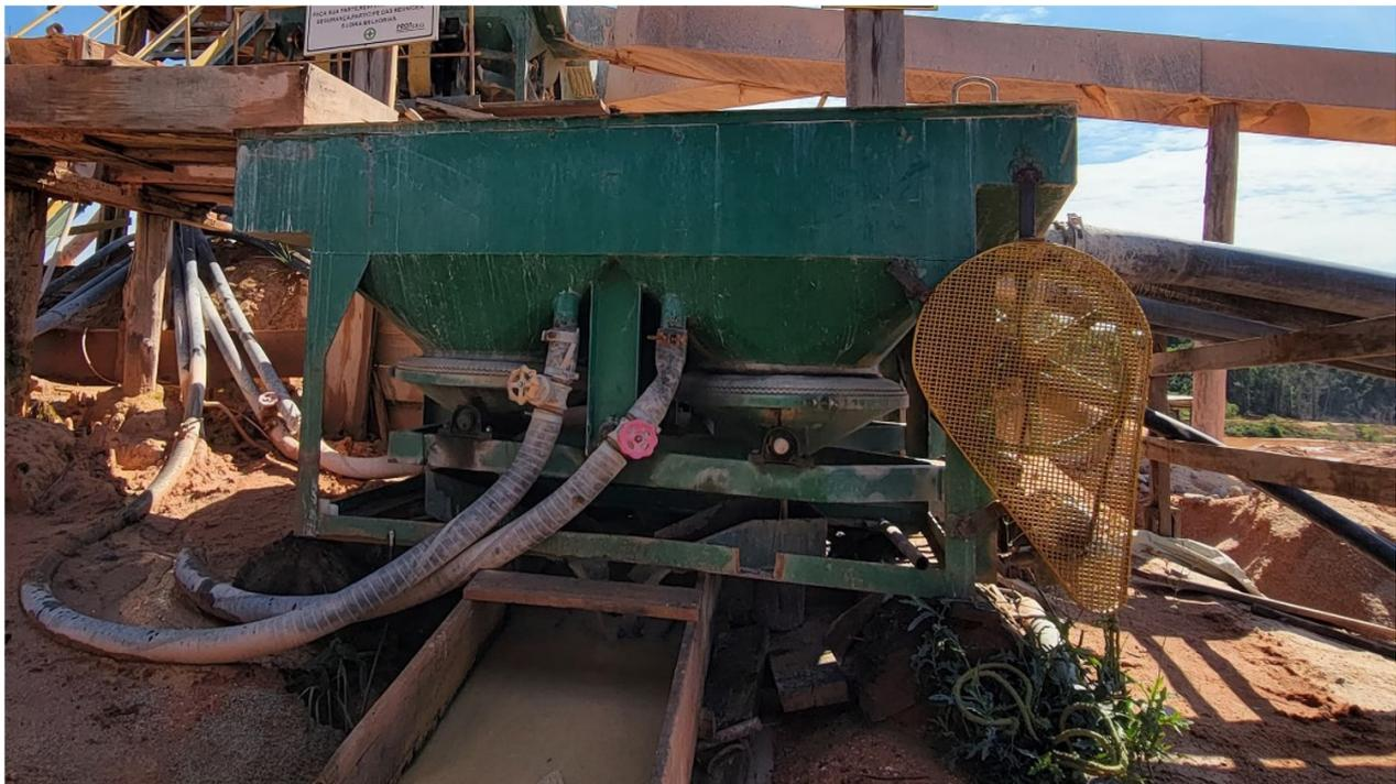
Figure 3. Twin cell Pan-American jig operating at São Francisco Mining.
