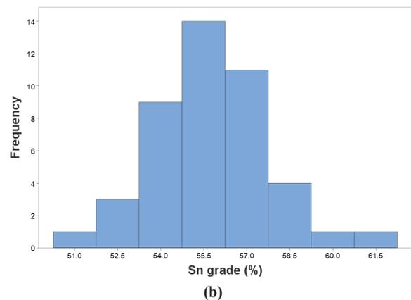
Figure 6. Frequency histogram of the daily Sn production (a) and grade (b) for one shaking table.
