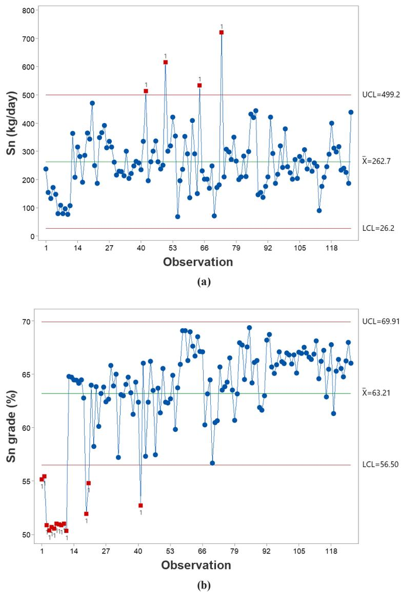
Figure 10. Control chart of the daily Sn production (a) and Sn grade (b) in the final concentrate produced for the jigs and shaking tables combined plants.
