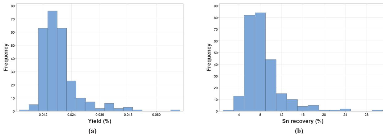
**Figure 4.** Frequency histogram of the daily yield (a) and Sn recovery (b) by jigs.
