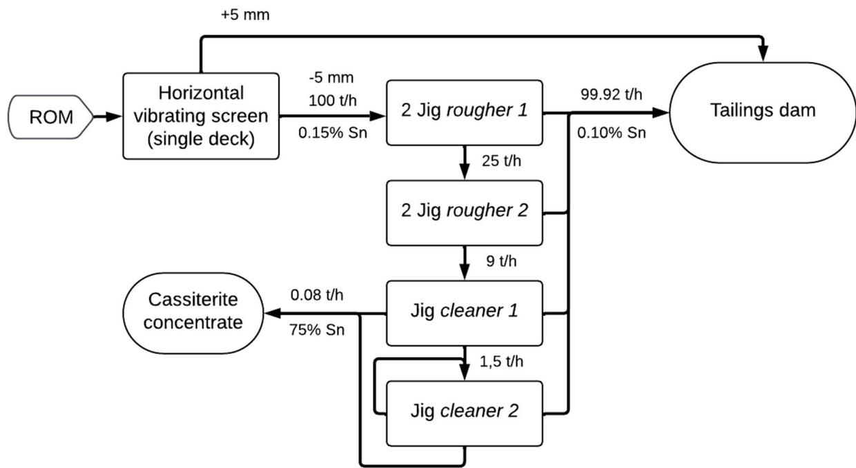
Figure 2. Cassiterite processing flowsheet before the shaking tables commissioning.
