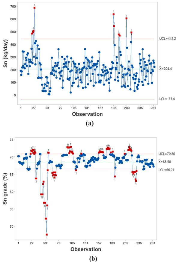
Figure 5. Control chart of the daily Sn production (a) and Sn grade (b) in the final concentrate produced by jigs.
