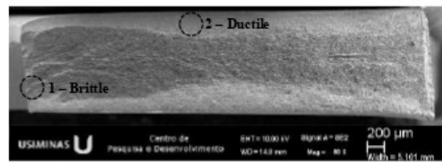
(b) Overview fracture - Charging Condition 3 – NaOH + 3 g/L \text{NH}_4\text{SCN}
