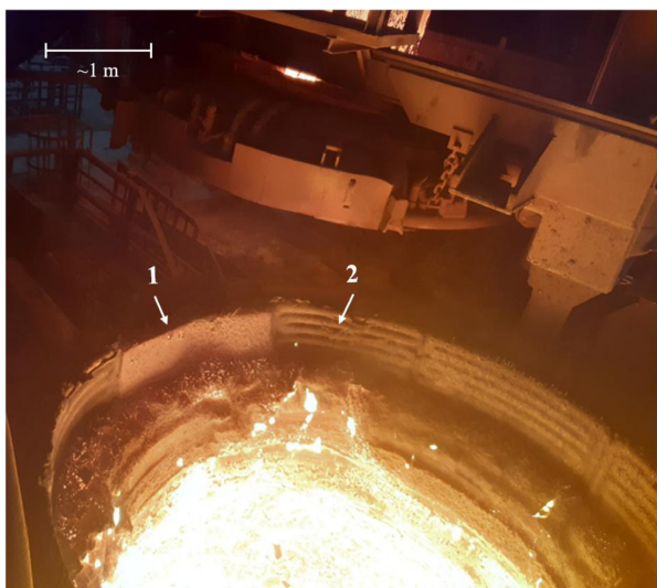
Figure 2. EAF upper sidewall with a refractory panel (1) replacing one of the water-cooled panels (2).
