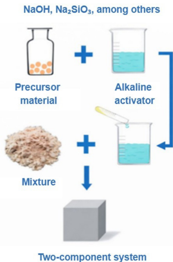
Figure 1. Schematic representation of the preparation process of two-part alkali-activated materials using a liquid activator solution. Adapted from [16].
