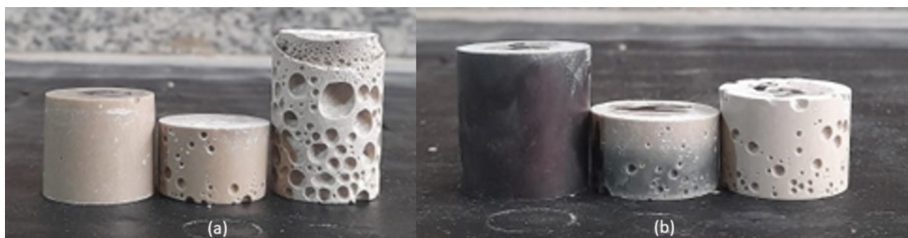
Figure 1. Specimens after demolding. (a) MK-based group; (b) MK+GBFS-based group.
