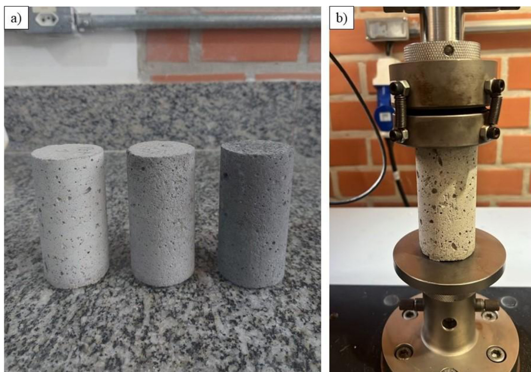
Figure 1. (a) Cylindrical mortar specimens after curing; (b) Compression test setup.
