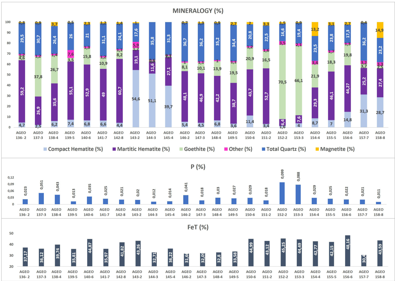
Figure 2. Summary of characterization results from the different mine face samples.
