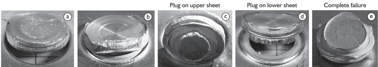
Figure 7. Fracture modes in shear tensile test: a) through weld with circumferential crack, b) plug pull-out with nugget tearing, and c) plug pull-out with back plug variations.
