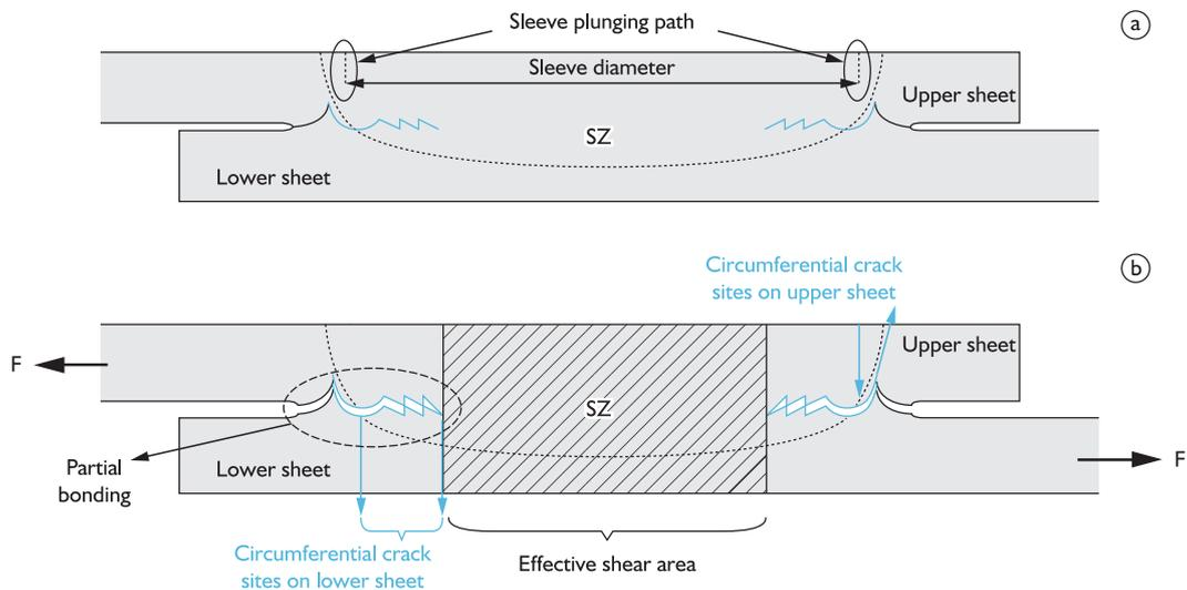
Figure 8. Schematic drawing showing the fracture development of FSpW joints under shear tensile loading. Notice that the joint dimensions are out of proportion for clarity.
