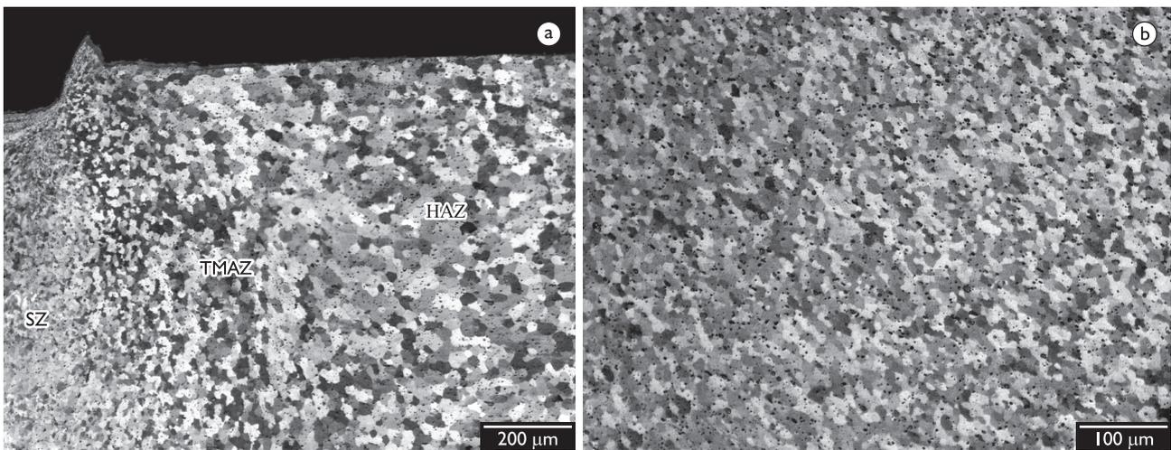
**Figure 4.** Optical micrographs obtained by electrolytic etching using Barker solution and viewed with polarized light showing details of: a) distorted grains in the TMAZ, and b) refined microstructure in the SZ.
