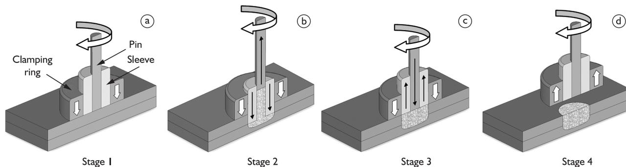
**Figure 1.** Schematic representation of the FSpW/sleeve plunge process: a) clamping and spindles rotation, b) sleeve plunges into the sheets while pin moves upwards, c) spindles retract back, and d) withdrawal of welding head.
