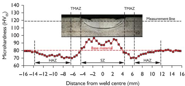
**Figure 5.** Microhardness profile measured in the middle of the upper sheet at the cross section of a FSpW joint welded according to the welding condition number 10 (2900 rpm / 3 s).
