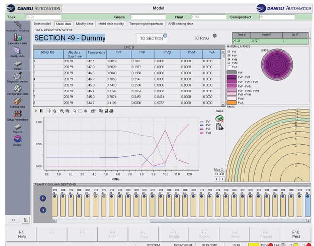
**Figure 4.** Distribution of different phases along radius of the bar.
