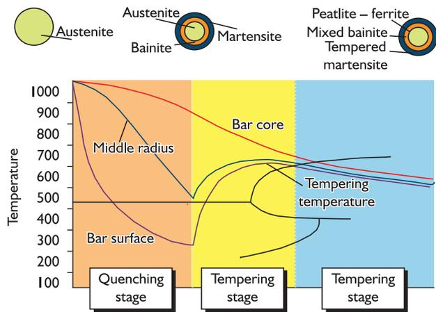
Figure 2. Quenching and self-tempering.
