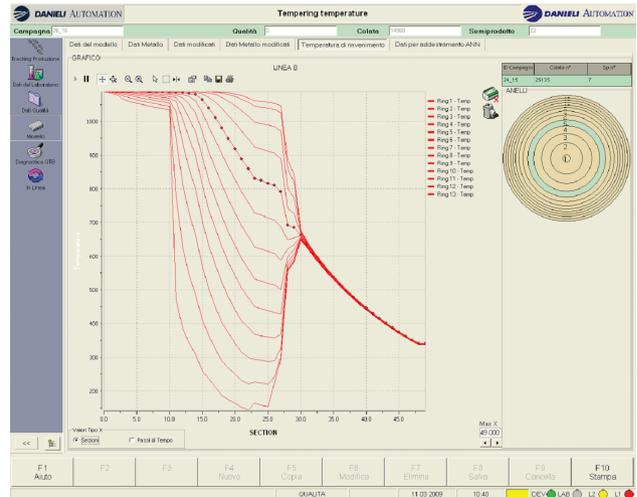
**Figure 3.** Temperature distribution at different annular sections of bar during and after quenching.
