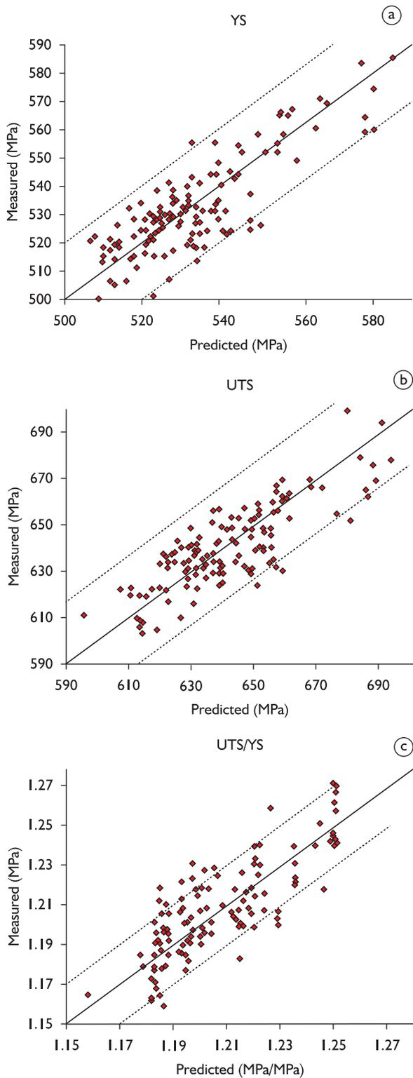
**Figure 6.** Comparison between actual vs. predicted values of a) YS; b) UTS, and c) UTS/YS.
