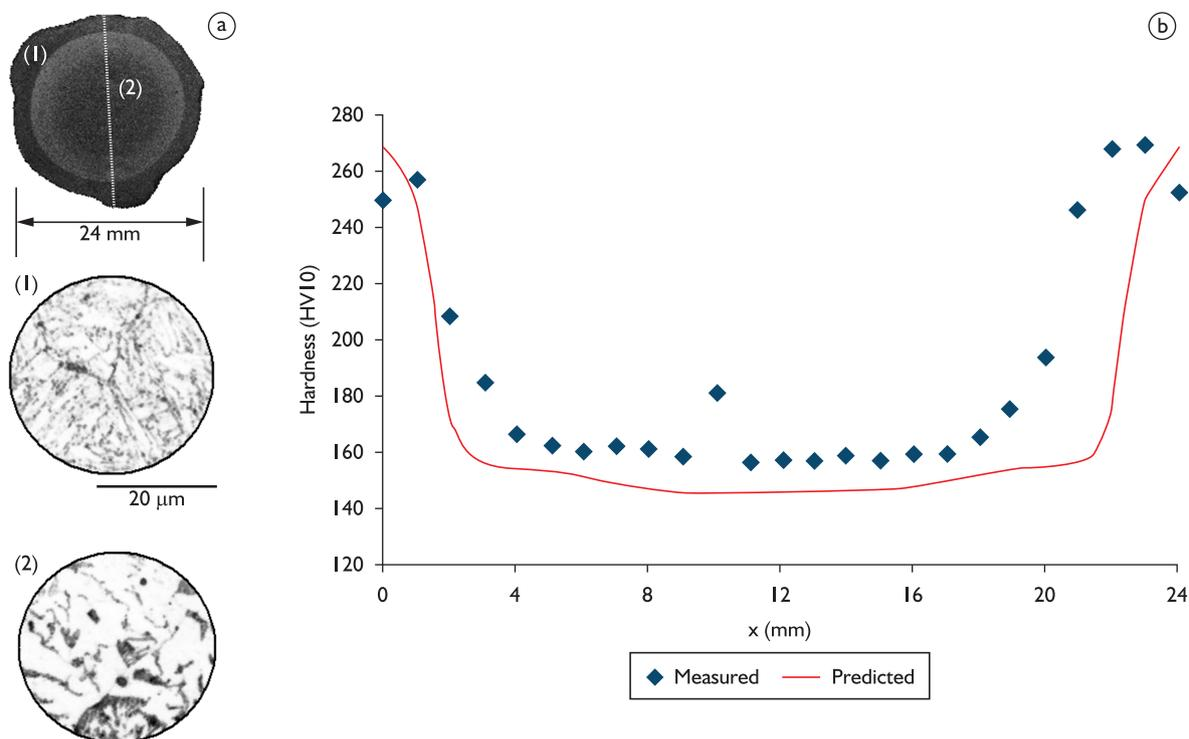
**Figure 5.** Comparison between actual and predicted structure & properties of  $\Phi$  24 mm rebar.
