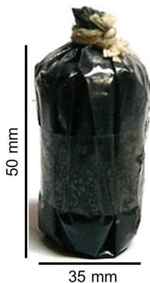
**Figure 3.** Self-reducing bag of mill scale and petroleum coke.
