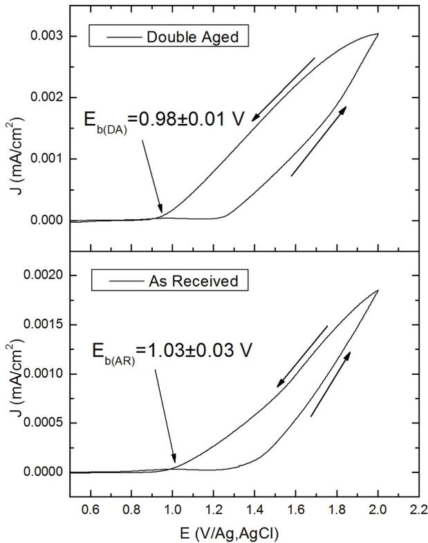
**Figure 1.** Cyclic voltammograms of double aged and as received Inconel 718 surfaces exposed to sodium chloride aqueous solution. Scan rate = 5 mV/s.
