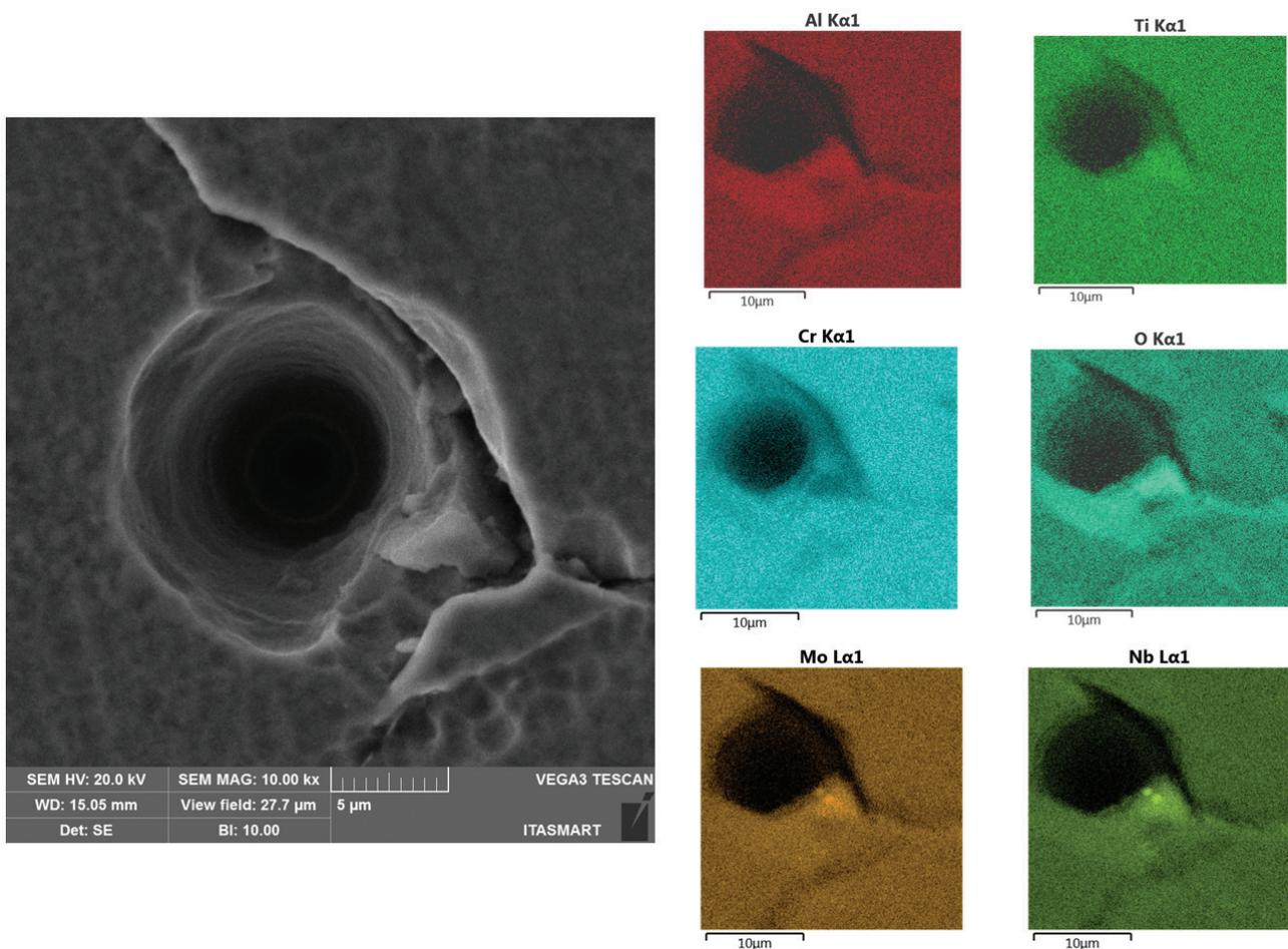
**Figure 5.** Image of a pit in Inconel 718 double aged, and the map scan of main elements around this pit.
