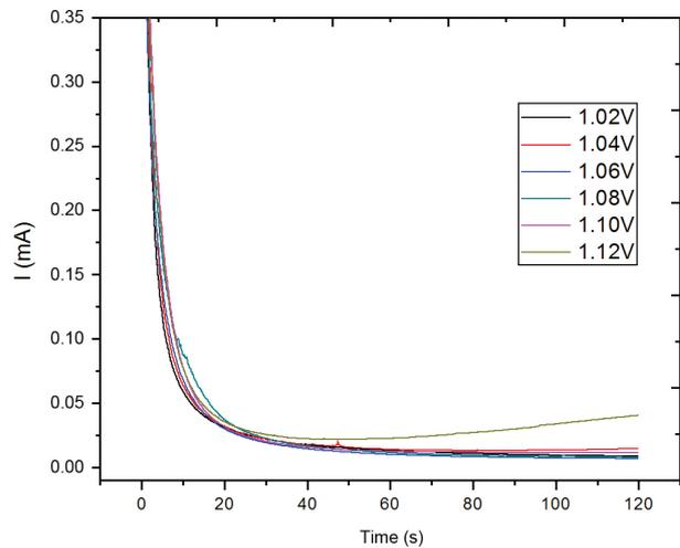
**Figure 3.** Chronoamperometric tests for double aged Inconel 718 surfaces exposed to chloride containing aqueous solution.
