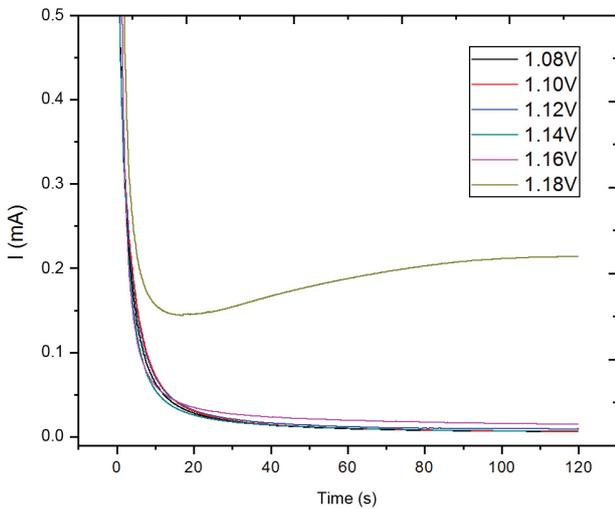
**Figure 2.** Chronoamperometric tests for as received Inconel 718 surfaces exposed to chloride containing aqueous solution.
