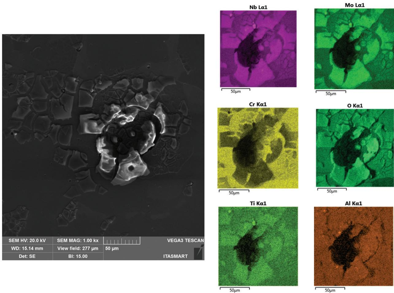
**Figure 4.** Image of a pit in Inconel 718 as received, and the EDS map scan of the main elements around this pit.
